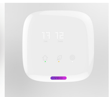
Figure 55. Final interface, with RGB LEDs that indicate air quality, and more intuitive icons
