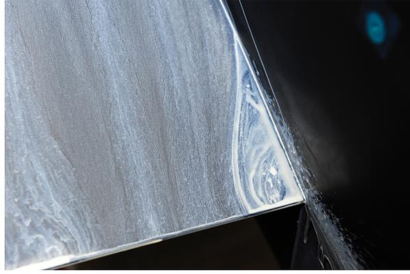
**Figure 2.3:** Corner separation on the trailing edge of a DLR-F6 wing connected to a fuselage at angle of attack of 5.0 degrees, image from Kegrise et al. [15].
