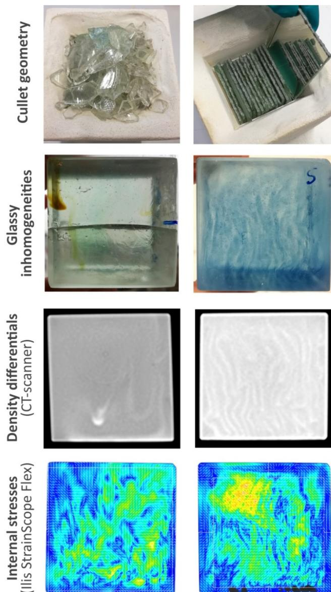
Figure 5. Glassy inhomogeneities as these resulted from 1) a variety of different soda-lime glasses: left column, sample no. 10, and 2) a metallic coating: right column, sample no.5. In the CT-scan images, white colour corresponds to higher density.
