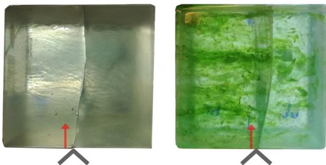
Figure 11. Side view of samples 10ii (left) and 11ii (right), showing the upward direction of the force and the perpendicular to the force- zones of inhomogeneities.
