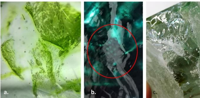
Figure 7. a) Glassy inhomogeneities (B2) due to the heat-resistant frit in sample 9. b) Sample 8, incompletely molten frit, retaining the pattern of the initial coating. c) Presence of different glass type in sample 10, leading to cracking (B3).
