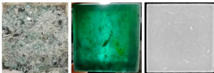
Figure 6. Glassy inhomogeneities in samples no.7. Relation of the density gradient as seen at the CT-scan (right) to the cullet size and contamination (left).
