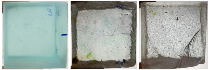
Figure 8. Bubble content increases with the decrease of cullet size. From left to right, samples no. 1, 10 and 11.
