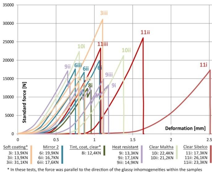
Figure 10. Splitting test results: force versus deformation graph
