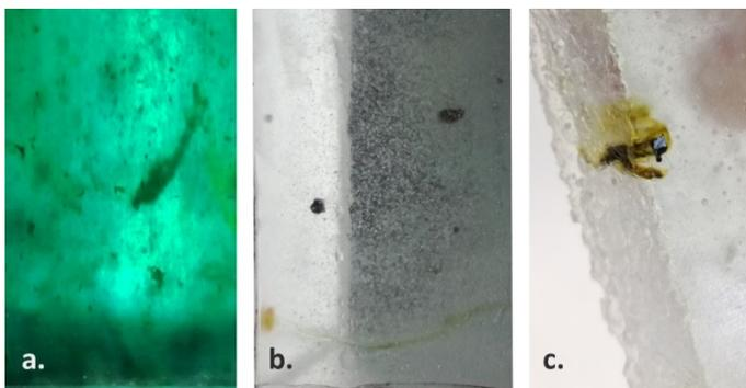
Figure 4. Crystalline inclusions observed in the cast specimens: a) Sample no. 7, defect A1. b) Sample no. 11, defect A1. c) Sample no. 11, defect A2.
