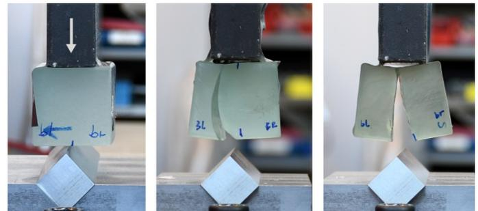
Figure 9. Left: splitting test set up. Middle: sample 6iii. Right: sample 10ii. The meso-structure of the specimens seems to affect the path of the crack.
