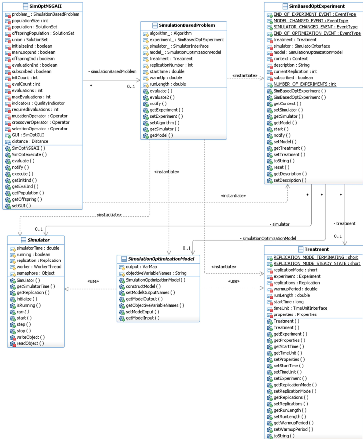
FIGURE 45 EXTENDED UML CLASS DIAGRAM OF SIMULATION AND OPTIMIZATION INTERACTION
