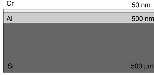
Figure 3.9: A schematic plot showing the deposited layers using EBPVD as a back-contact. The top Cr layer protects the Al from being etched by KOH.
