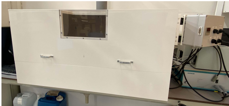
Figure A.10: The Autolab setup sits inside the white box, creating a safe work environment to place the cell setup filled with chemicals.
