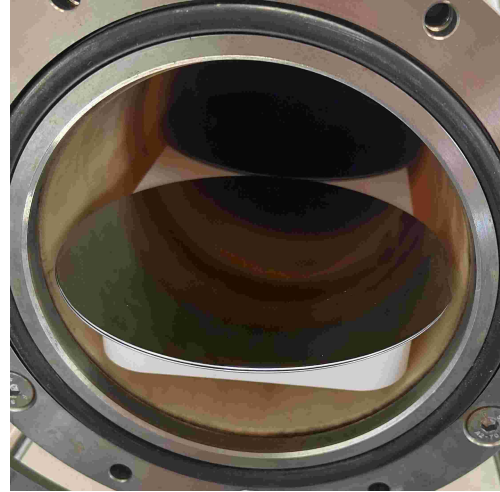
Figure 3.6: A four inch wafer fits in the load-lock. A protective wafer is placed on the bottom to prevent any residue material from the white ceramic to diffuse through.
