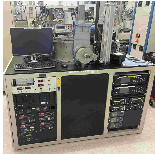
Figure A.5: The AMOR setup. The load lock is the round tube at the front and is used to enter the wafer holders. The wafers are put in one by one.
