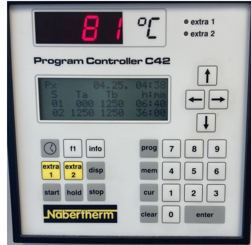
Figure A.7: The control panel of the tube furnace, with three time periods with corresponding temperatures to be set: ramp up, continuous and ramp down temperature.
