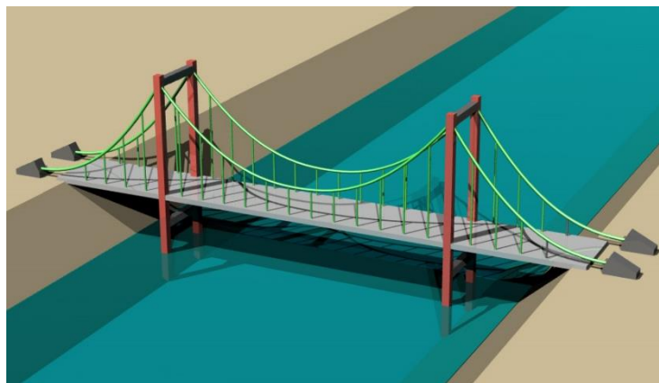
Figure 7.10: Tensile (green) and compressive (red) forces in a typical suspension bridge construction
