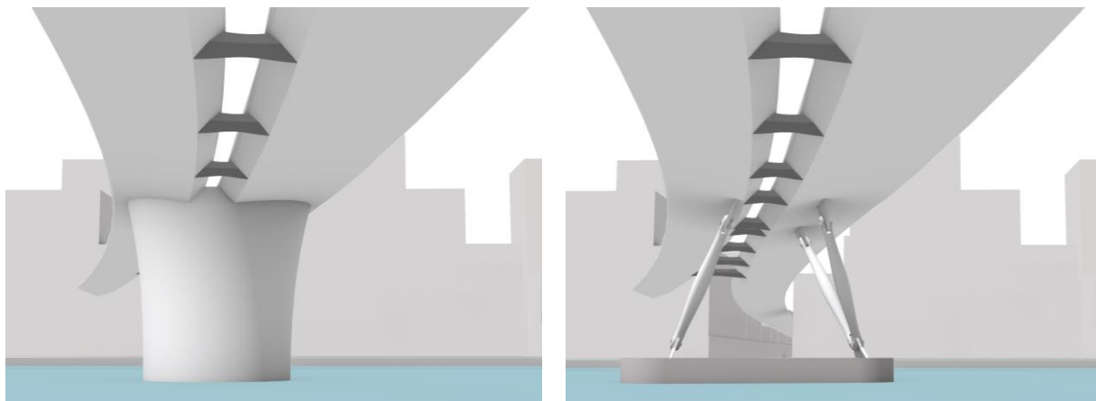
Figure 11.20: Solid supports will interrupt the flowing lines as created by the bridge decks (left) Sleeker support structures leave the flowing lines intact (right)
