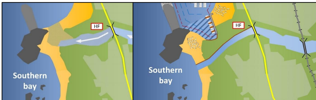
Figure H-2: Current position of the river (l) and the redesigned channel (r)
