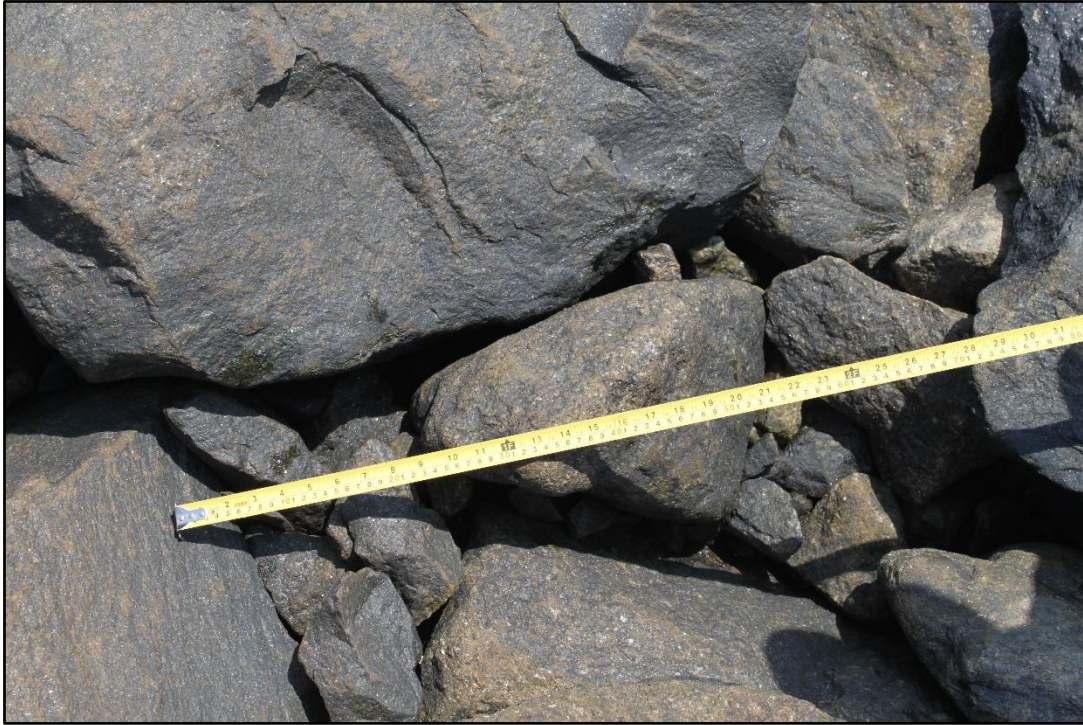
Figure R-1: Small stones in between big stones
