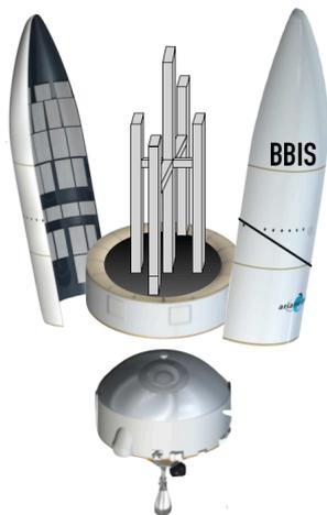
Figure 12.2: Adaptor Structure Inside of Launcher.
