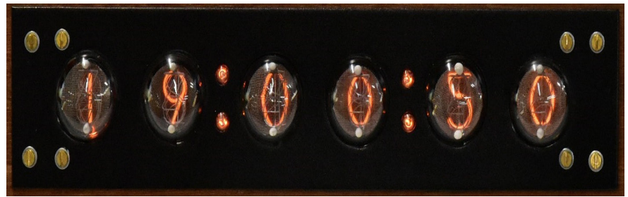
Figure 11. Electronic clock, which uses Nixie-tubes, displaying '19:00:50'
