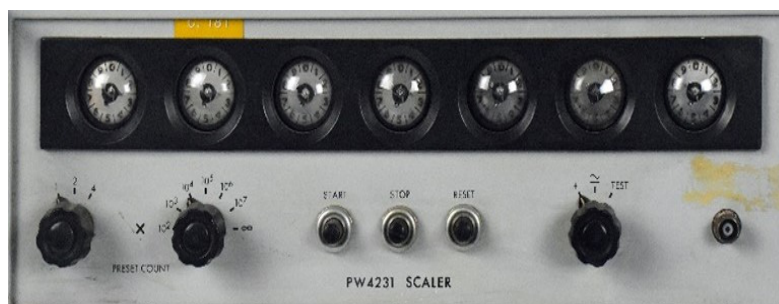
Figure 9. Philips Scaler 4231 using this special ZM 550 tube
