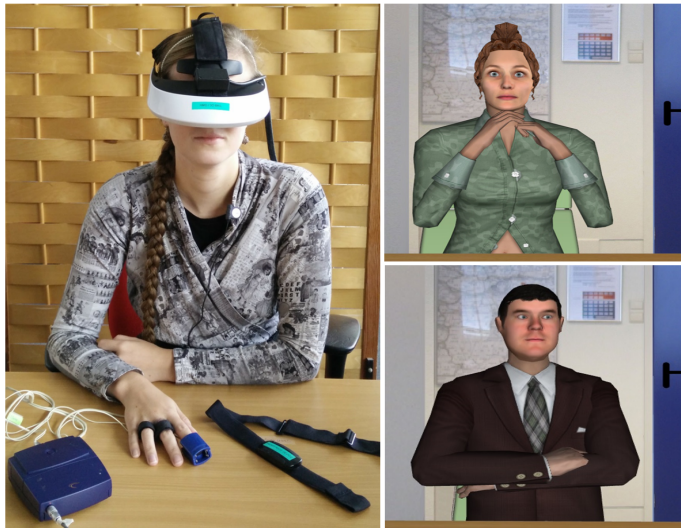
Figure 4.5: (Left) Physical equipment participant used during the experiment: head mounted display (HMD) with head tracker, heart rate monitoring devices; Mobi 8 (finger clips), Zephyr HXM (chest band) and a microphone. (Right) The female and male interviewers with different body postures and eye gaze seen by the participant
