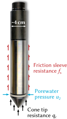
Figure 1.3: An example of a cone penetrometer (CPT) and the measurements it collects.
