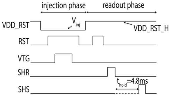
Fig. 2. Timing diagram of the feed forward measurement
