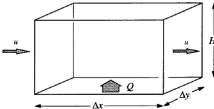
Figure 2.1: Graphical representation of the box model. (Seinfeld and Pandis, 2016)
