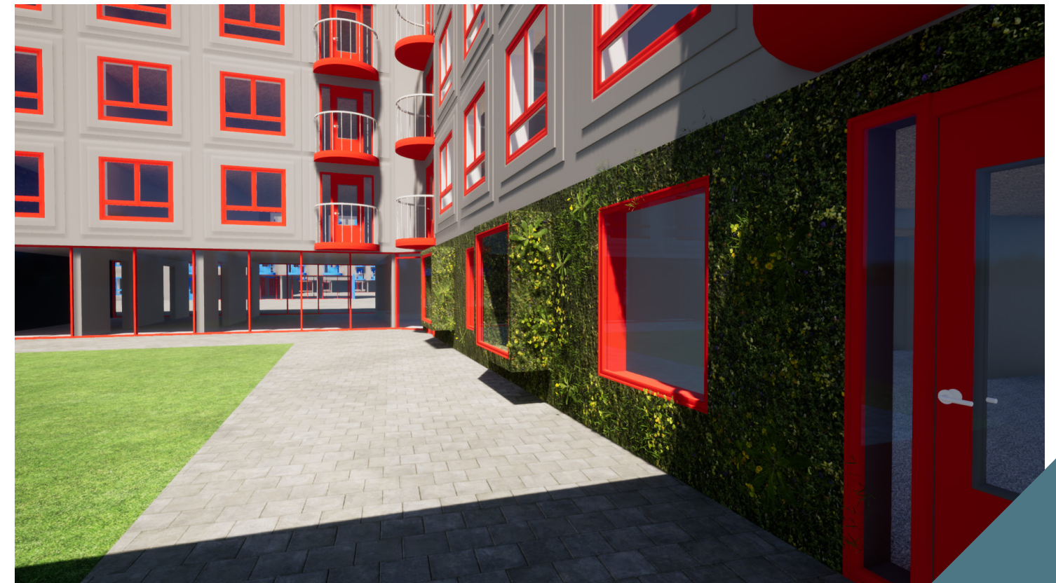
Ground floor (semi-public functions) with new green facade and new windows. This option has the most benefits. The green facade has a positive effect on increasing the biodiversity, air quality and health and well being of people. It also increases the investment value.
