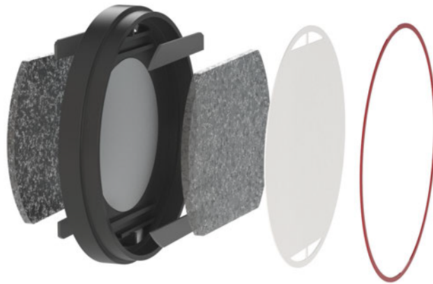
figure 49 Exploded view of electrolysis cell of concept #1
