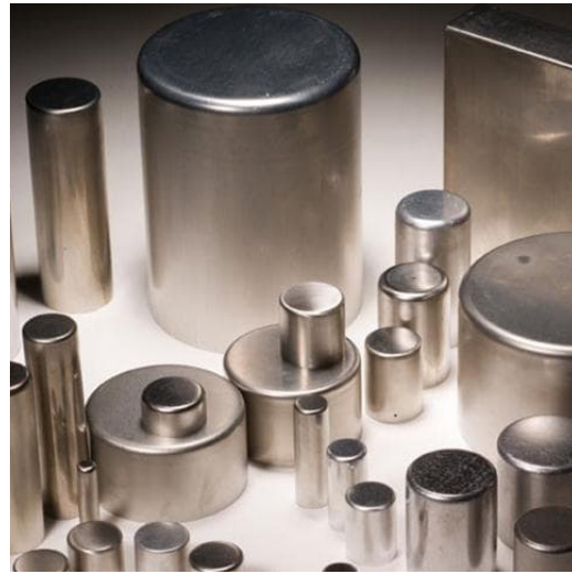
figure 43 Example of deep drawn shapes
