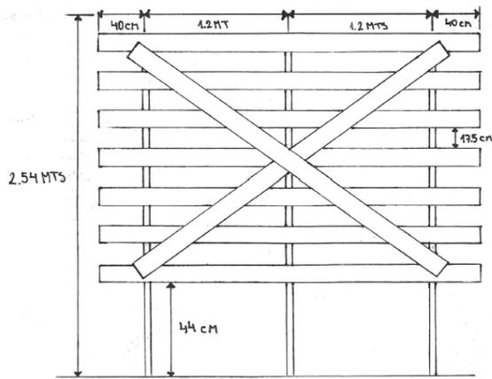
Figure 3.6: Front view and dimensions of one part of the snow fence.
