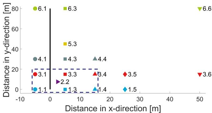
Figure 3.8: Sketch of the snow stakes and fence at Tascadero. The black line represents the fence, the numbered marks indicate the stake locations. The stakes are coloured such that one color represents one line of stakes.
