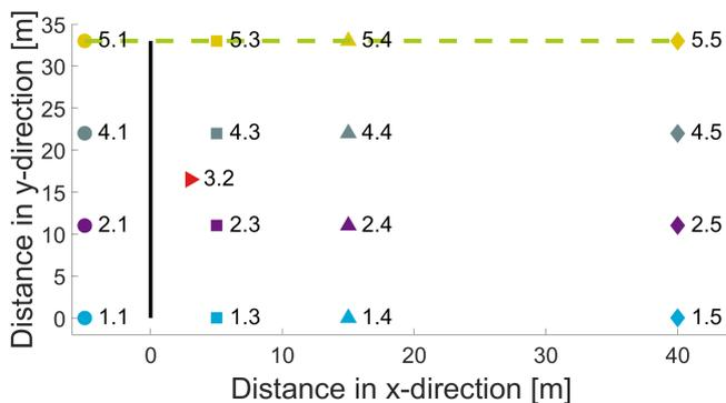
Figure 3.9: Sketch of the snow stakes and fence at Llano. The black line represents the fence, the numbered marks indicate the stake locations. The stakes are coloured such that one color represents one line of stakes.
