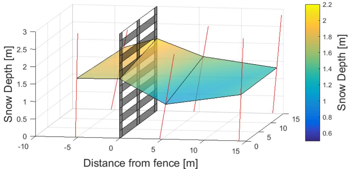
Figure 3.16: Snow depth in Tascadero on August 26, 2017 in 3D representation
