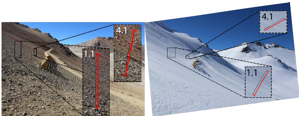
Figure 3.14: Example for method 2 using the photo taken on June 10, 2017. The level of zooming is different and therefore the red lines indicating the length of pnghe stakes do not represent the real length in the image, which is 3.00 meters for both stakes.
