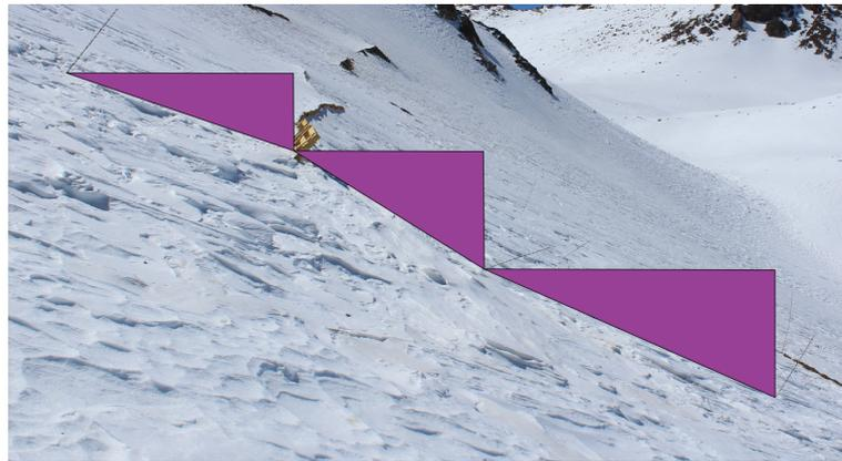
Figure 3.17: Example of the triangles used to calculate the angle between stakes and stakes/fence on August 30, 2017
