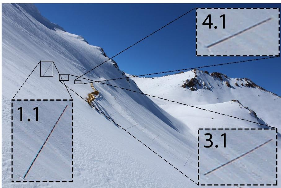
Figure 3.13: Example for method 1 using the photo taken on June 10, 2017. Each stake has a length of 3 meter.
