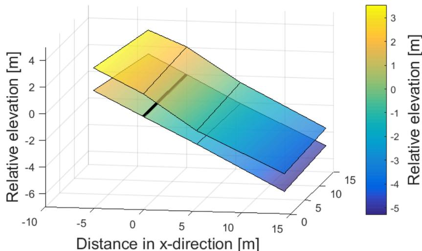
Figure 3.15: A plane of the ground surface without snow and a plane of the snow surface are shown for Tascadero on August 26, 2017. The thick black line marks the bottom of the snow fence.
