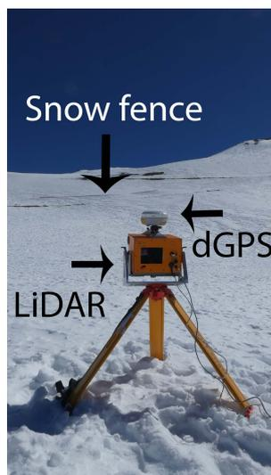
Figure 3.11: Taking LiDAR measurements at Tascadero on August 30, 2017
