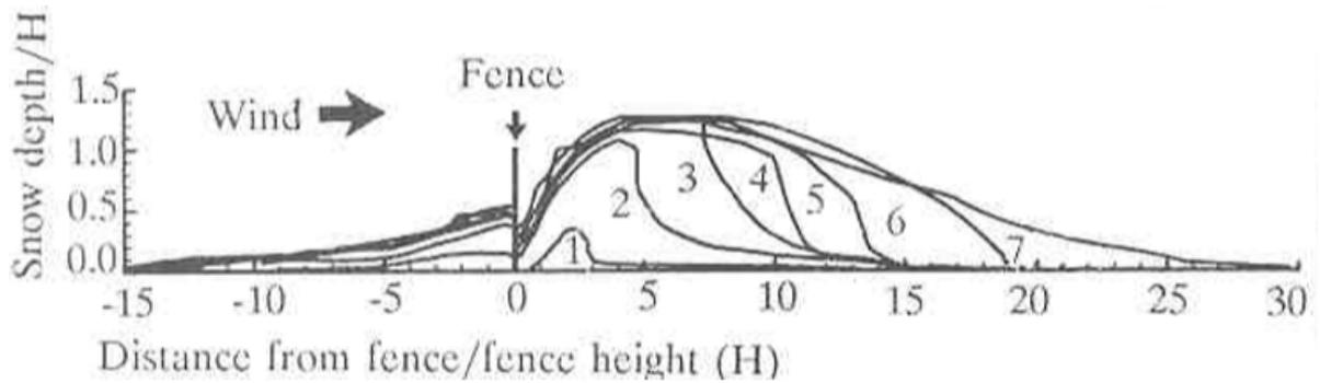
Figure 2.1: A sketch of the different stages of the effect of a snow fence with 50% porosity. This image is taken from the technical report of R.D. Tabler [18].
