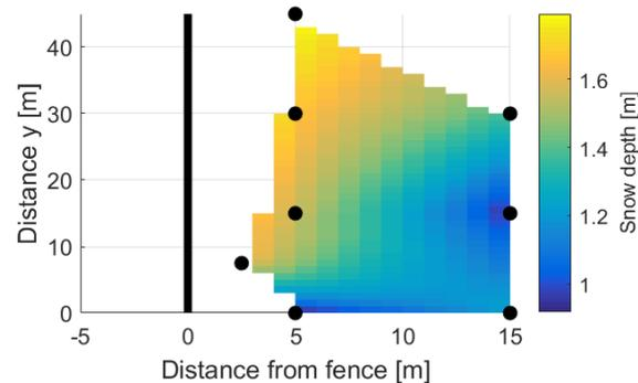
Figure 4.2: Resulting snow depth using the LiDAR data. The values are obtained by calculating the difference between the LiDAR data on March 15, 2017, when no snow was present and on August 30, 2017.
