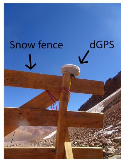
Figure 3.12: An example of dGPS measurements done in Llano on October 5, 2017. Here, the exact location of the end of the fence is measured. The stakes locations are measured similarly, with the pole of the dGPS device placed on the ground.
