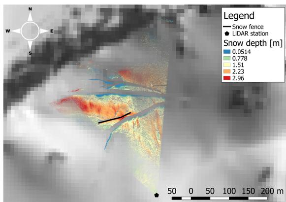
Figure 4.1: The resulting snow depth from two LiDAR datasets on August 30, 2017, covering a Landsat image obtained on September 1, 2017. Because the angle between the LiDAR station and the roads around the snow fence are small the roads are visible because the data is lacking. The LiDAR image was provided by Nicole Schaffer (CEAZA).
