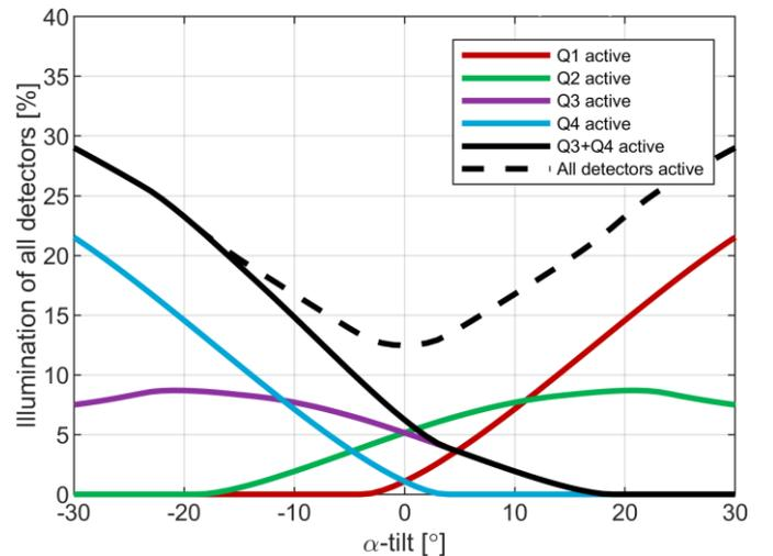
Fig. 3. The illumination percentage of the EDS detector, which shows the percentage of the total surface area of the detector that is used to detect characteristic X-rays, at different  $\alpha$ -tilt angles, and for different configurations of active detectors. Valid for the DENSSolutions double-tilt sample holder. Detectors Q2 and Q3 are shadowed by the cradle, detectors Q1 and Q4 are shadowed by the contact needles.
