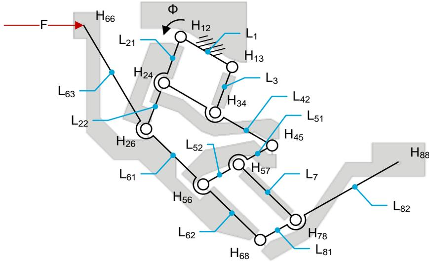
Fig. 18. The numbering of the hinges and links in the proof-of-principle mechanism.
