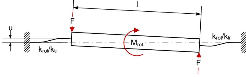
Fig. 21. The free-body diagram of a link that is connected to two flexures with an equilibrium between the moment  $M$  induced by the rotational stiffness in the hinges and the forces  $F$  as a result of the transverse stiffness in the hinges.
