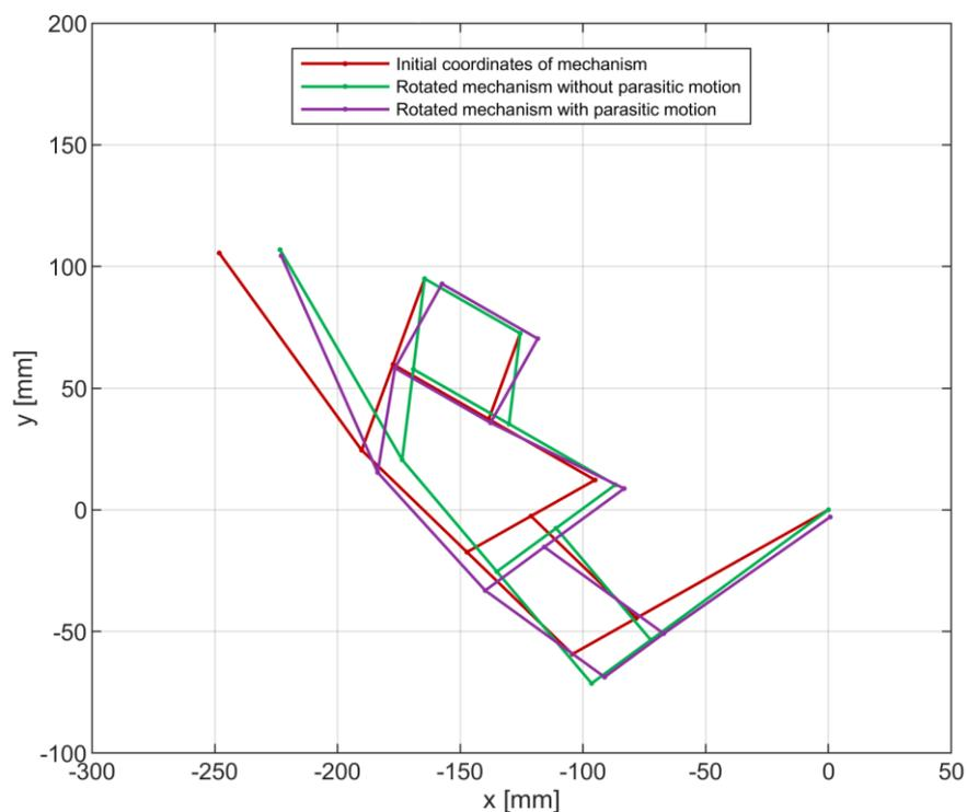
Fig. 20. The effect of hinge shift on the kinematics of the mechanism. The hinge shift is exaggerated for illustrative purposes, in reality the hinge shift is 10 times as small. It can be seen that the hinge shift is quite large everywhere, but the effect on the RCM and the actuation location is marginal. The hinges in the mechanism are orientated in such a way that their effects cancel each other out.
