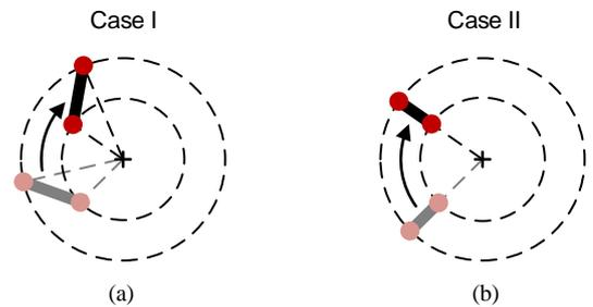
Fig. 5. The two cases in which a body can rotate around a point. (a) Case I, in which two points on a body are not collinear with the center of the concentric circles and where the circles can have arbitrary radii and (b) case II, in which two points on a body are collinear with the center of the concentric circles and the radii of the circles are not equal.
