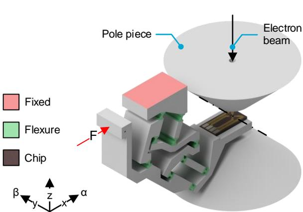
Fig. 12. An illustration of how a compliant RCM mechanism created with the novel RCM mechanism design strategy can be used in the sample holder. The mechanism is fixed at the top and actuated from the left.
