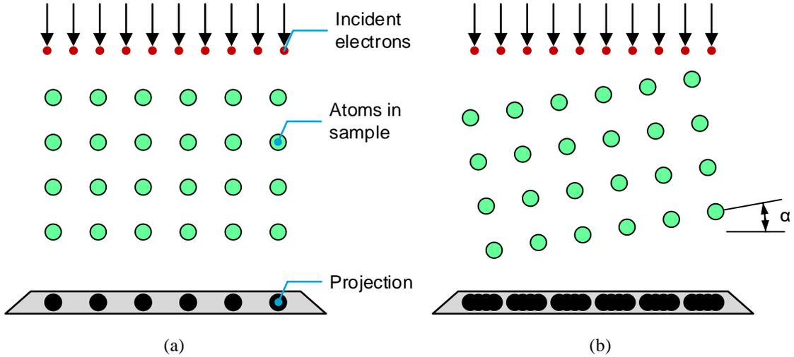
Fig. 8. The effect of rotating the sample with respect to the incident electron beam. (a) The crystal structure of the sample aligned with the incident electron beam. (b) The crystal structure of the sample misaligned with the incident electron beam.
