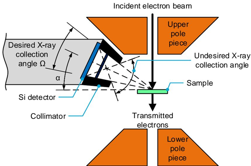
Fig. 6. A schematic drawing of the EDS detector in a TEM. Adapted from [2].
