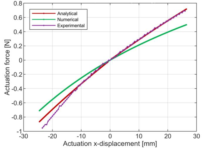
Fig. 16. Three force/displacement curves obtained by analytical, numerical or experimental analysis. The displacement range corresponds to a rotation of input link of  $\pm 13^\circ$ .
