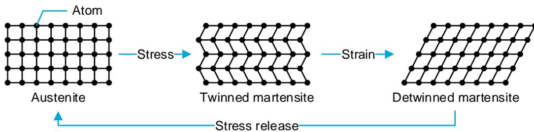
Fig. 15. The phase transformation of superelastic Nitinol as a result of stress and strain.
