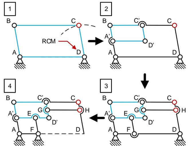
Fig. 10. The novel RCM mechanism design strategy. 1. The basis of the design strategy is an arbitrary four-bar mechanism, with its future RCM defined as point D. 2. The shape of the four-bar mechanism is scaled down into the corner of B. 3. Two links are added; link EF which is parallel to link AB that connects link AD with link A'D'. And link GH which is parallel to link BC that connects link CD with link C'D'. 4. Finally the constraint at D is moved to F and link FD is removed.
