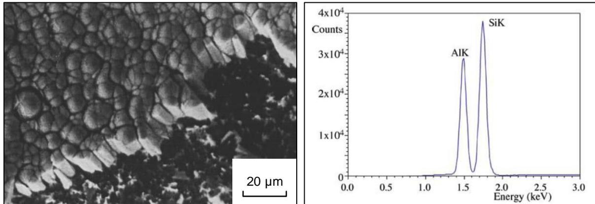
Fig. 4. (left) An image of Al evaporated onto a Si substrate and (right) its spectrum created with EDS. [2]
