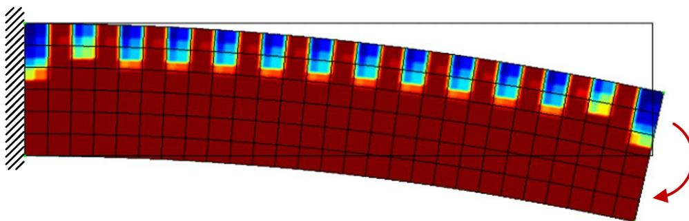
Fig. 17. A plot of the Young's modulus in a Nitinol beam when a moment is applied on the right side. The localization is shown, that occurs due to the local reduction of the stresses when a nearby node switches to the superelastic behavior.
