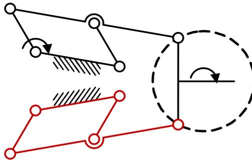
Fig. 14. Two of the three virtual center mechanisms used in concept 10 and depicted in black and red. By connecting the two mechanisms the RCM is defined.
