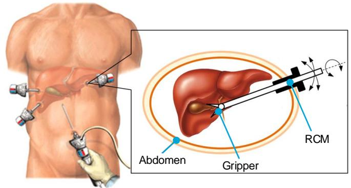
Fig. 1. An illustration of the use of a RCM mechanism in MIS. By having a RCM at the point where the surgical tool (in this case a gripper) enters the abdomen only a very small incision is required while the tool can still be manipulated inside the body. Adapted from [3].
