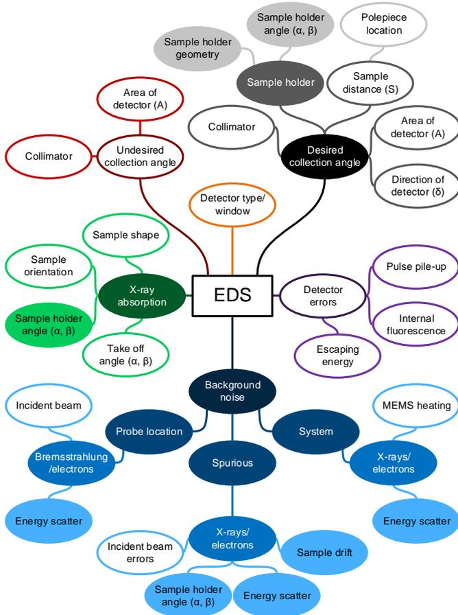
Fig. 2. A detailed overview of the EDS influences up to the point that the signal exits the detector and enters the electronics and data processing part. The overview shows through which paths the influences in the outermost bubbles have an effect on the performance of the EDS analysis. The influences and their paths that are relevant for the sample holder design are indicated by the solid bubbles.
