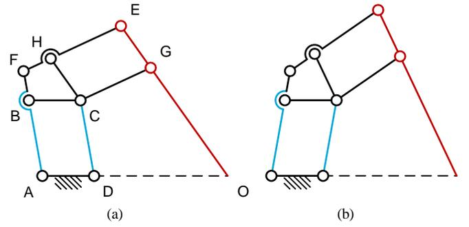
Fig. 9. A RCM mechanism that has input (in blue) and output links (in red) whose lengths are non-equal, and which are non-parallel. Two configurations are shown; (a) the initial and (b) the rotated configuration. Adapted from [24].
