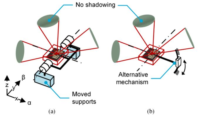
Fig. 5. (a) Optimization path I; reducing or changing the footprint of the current mechanism to make sure the tilting mechanism does not interfere with both the MEMS zone and the detector zones. (b) Optimization path II; using another type of RCM mechanism that does not interfere with the MEMS zone and the detector zones. A goniometer mechanism is shown here. For clarity only three out of four EDS detectors are illustrated.
