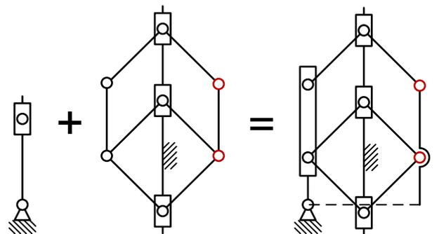
Fig. 10. An illustration of the strategy of combining a 1RIT mechanism and a RMTM to create a 1RIT RCM mechanism. By using a 1R mechanism and a RMTM mechanism a 1R RCM mechanism can be created. Adapted from [13].
