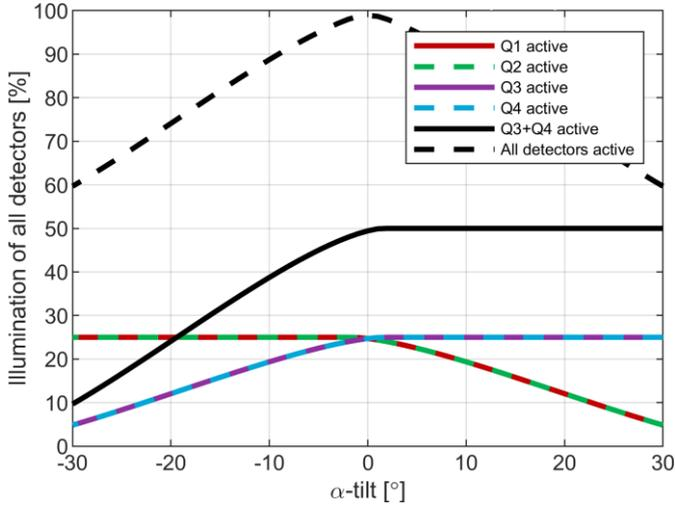
Fig. 7. The detector illumination as a function of  $\alpha$ -tilt for concept 1, 2 and 3. At  $0^\circ$  of  $\alpha$ -tilt the illumination goes up to 100%, which is a sevenfold increase in comparison with the current sample holder design. For larger  $\alpha$ -tilt angles this number drops down to a twofold increase in EDS illumination.
