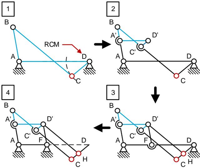
Fig. 11. The novel RCM mechanism design strategy with a more complex four-bar mechanism as its starting point. In this case the hinge points E and G of Fig. 10 are merged with D'.
