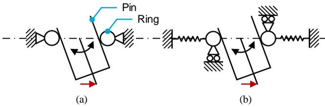
Fig. 3. (a) The planar version of a pin-in-ring joint, which needs play in between the pin and the ring to be able to rotate. (b) The compliant version of a pin-in-ring joint that does not need play to be able to rotate and can be considered a RCM mechanism of the compliant mechanisms class.
