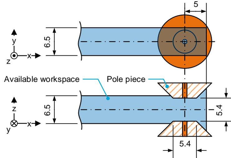
Fig. 7. The space available for the sample holder and tilting mechanism.
