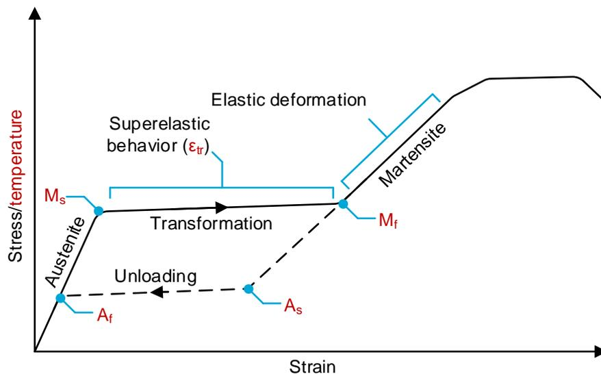
Fig. 16. The stress/strain curve of Nitinol with the transformation temperatures; austenite finish temperature ( $A_f$ ), austenite start temperature ( $A_s$ ), martensite start temperature ( $M_s$ ) and martensite finish temperature ( $M_f$ ).
