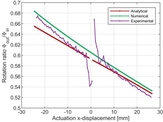
Fig. 18. The rotation ratio  $\Phi_{out}/\Phi_{in}$  as a function of the actuation x displacement. Obtained by analytical, numerical or experimental analysis. The displacement range corresponds to a rotation of the input link of  $\pm 13^\circ$ .
