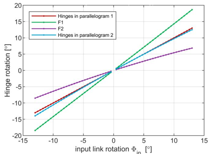
Fig. 17. The individual hinge rotations when the input link of the proof-of-principle mechanism is rotated over a range of  $\pm 13^\circ$ . For identification of the hinges see Fig. 14a.
