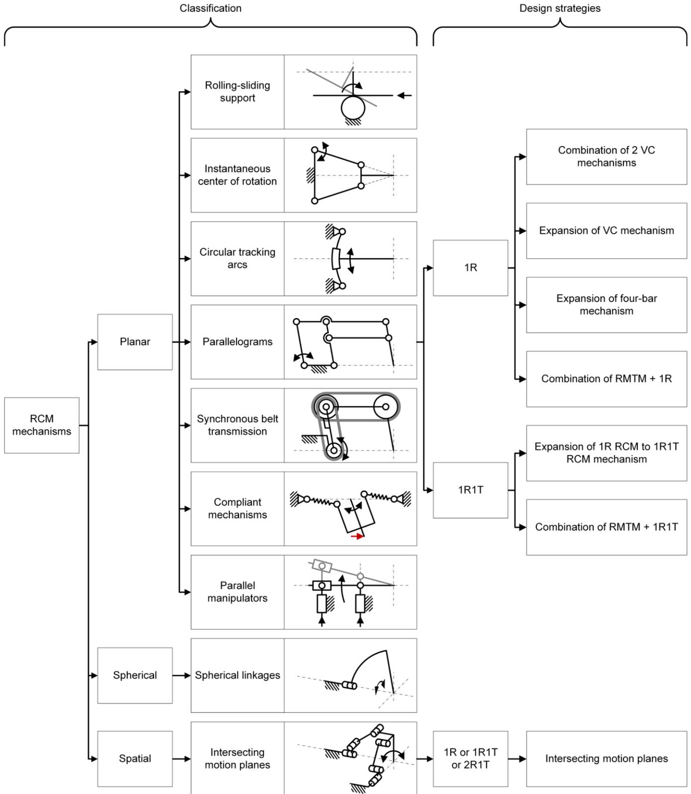
Fig. 2. An overview of the novel classification and design strategies for RCM mechanisms. The different RCM classes belong to the planar, spherical or spatial mechanisms group. For every class an example mechanism is shown, black arrows indicate movement, red arrows indicate forces. For two classes (the parallelograms and intersecting motion planes classes) design strategies exist which are subdivided by the amount of rotational (R) and translational (T) degrees of freedom.
