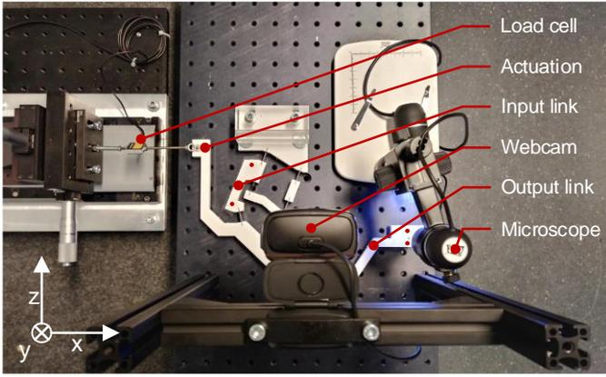
Fig. 15. An overview of the measurement setup with its different components. The proof-of-principle mechanism is actuated on the left side using a micro positioning stage. A webcam and a microscope are used to track dots on the mechanism and obtain the required data.
