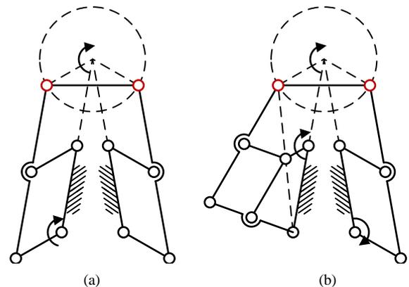
Fig. 6. Two RCM mechanism based on case I, created by using two VC mechanisms; one (a) created with two identical VC mechanisms and another one (b) created with two different VC mechanisms. The points (hinges) that describe circular motion are indicated in red.
