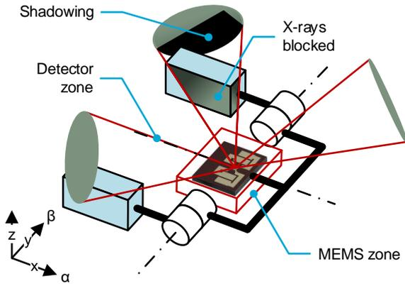
Fig. 4. An illustration of the RCM mechanism that facilitates the  $\beta$ -tilt in the DENSolutions double-tilt sample holder. The mechanism does not interfere with the MEMS zone, but it does interfere with the detector zones, blocking X-rays from reaching the EDS detector. For clarity only three out of four EDS detectors are illustrated.
