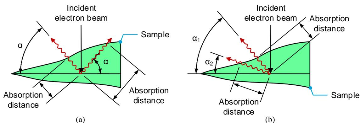
Fig. 5. The influence of (a) sample shape and (b) sample orientation, sample holder angle and take-off angle on the amount of absorption in the sample. Adapted from [2].
