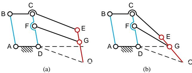
Fig. 8. Two variations on the standard double-parallelogram RCM mechanism with its input links in blue and its output link in red. (a) The standard mechanism which has the RCM property and (b) a mechanism with a rotated output link with respect to its input links which has lost its RCM property.
