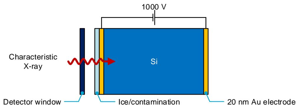
Fig. 2. A schematic overview of a Si detector. Adapted from [2].
