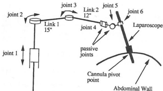
Fig. 4. An example of a mechanism from the passive RCM mechanisms class. The RCM is defined by the support of the abdominal wall. [16]
