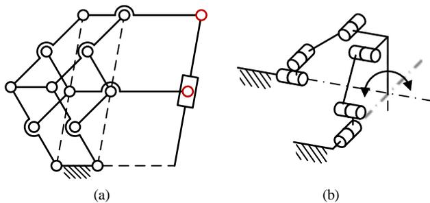
Fig. 11. (a) A 1R RCM mechanism (dashed lines) that is expanded to a 1R1T RCM mechanism. (b) A 1R RCM mechanism based on intersecting motion planes. The output link has a parasitic translation through its RCM when it is rotated.
