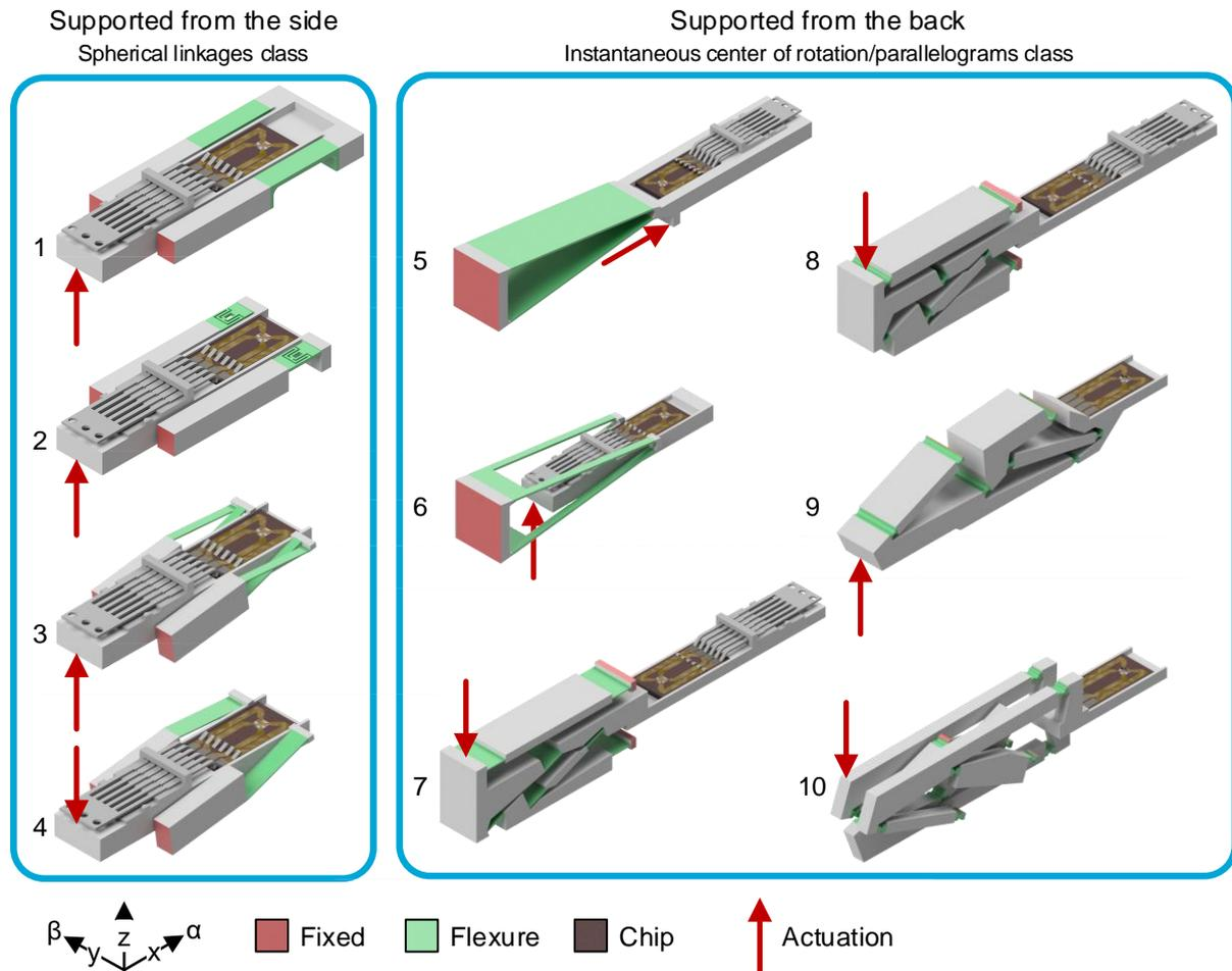
Fig. 10. The various concepts for the tilting mechanism in the DENSSolutions double-tilt sample holder that have been developed and evaluated.
