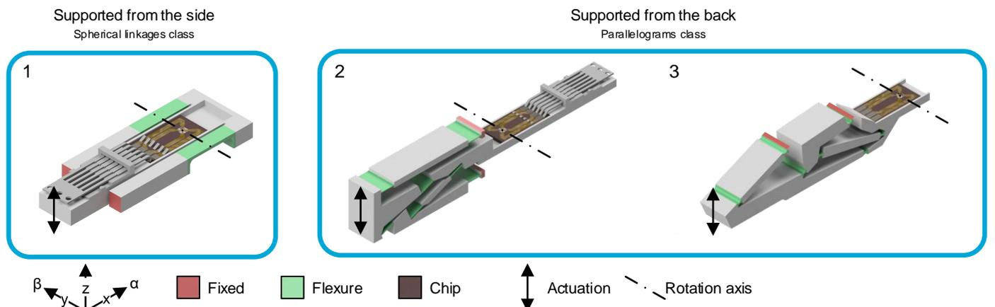
Fig. 6. Tilting mechanism concepts. The concepts can be divided into two groups; (left) concepts that replace the conventional revolute joints in the DENSolutions sample holder with flexures so that the MEMS chip is supported from the side, or (right) concepts that support the MEMS chip from the back, creating more space around the MEMS chip. The first group consists of RCM mechanisms from the spherical linkages class and the second group consists of RCM mechanisms from the parallelograms class.
