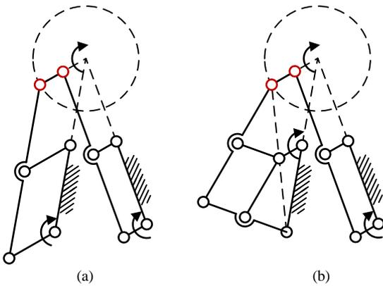
Fig. 7. Two RCM mechanism based on case II, created by using two VC mechanisms; one (a) created with two identical VC mechanisms and another one (b) created with two different VC mechanisms. The points (hinges) that describe circular motion are indicated in red.
