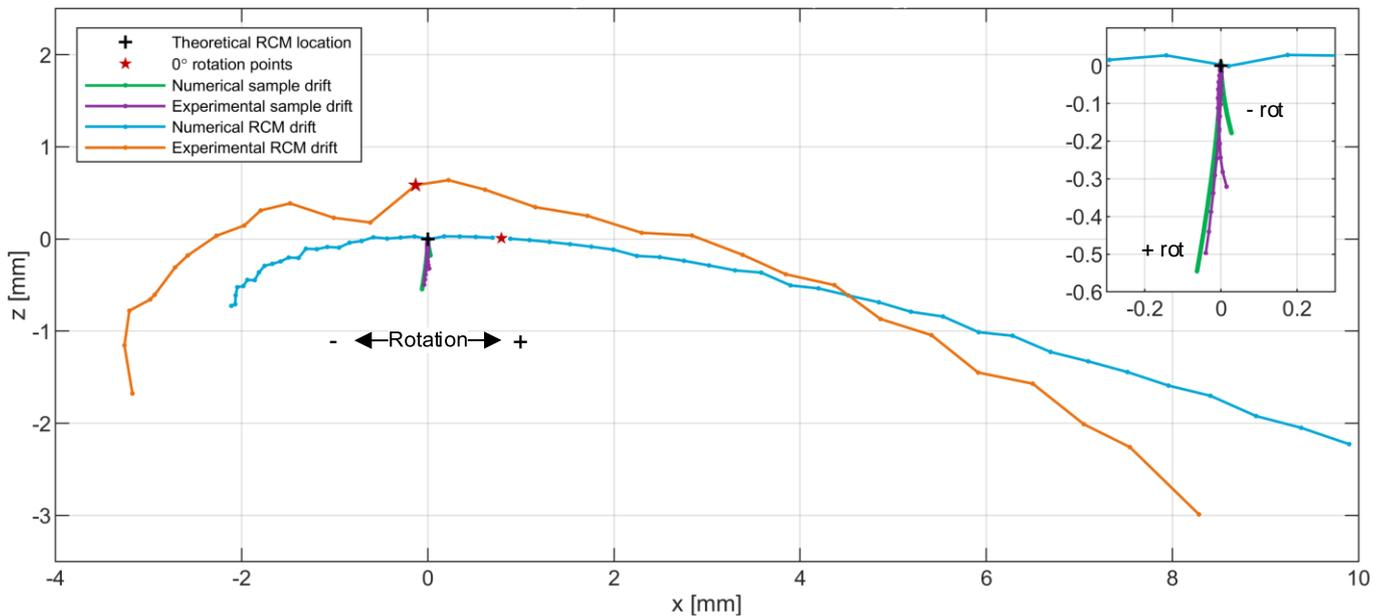
Fig. 19. The offset and drift of the RCM and the sample, for an input link rotation range of  $\pm 13^\circ$ . The sample drift as a result of positive and negative rotation are indicated. For the RCM drift curves, the part to the left of the  $0^\circ$  rotation point is a result of negative rotation and to the right is a result of positive rotation.
