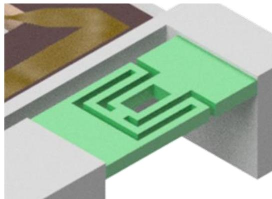
Fig. 11. The inverse lamina emergent torsional (I-LET) joint used in concept 2.
