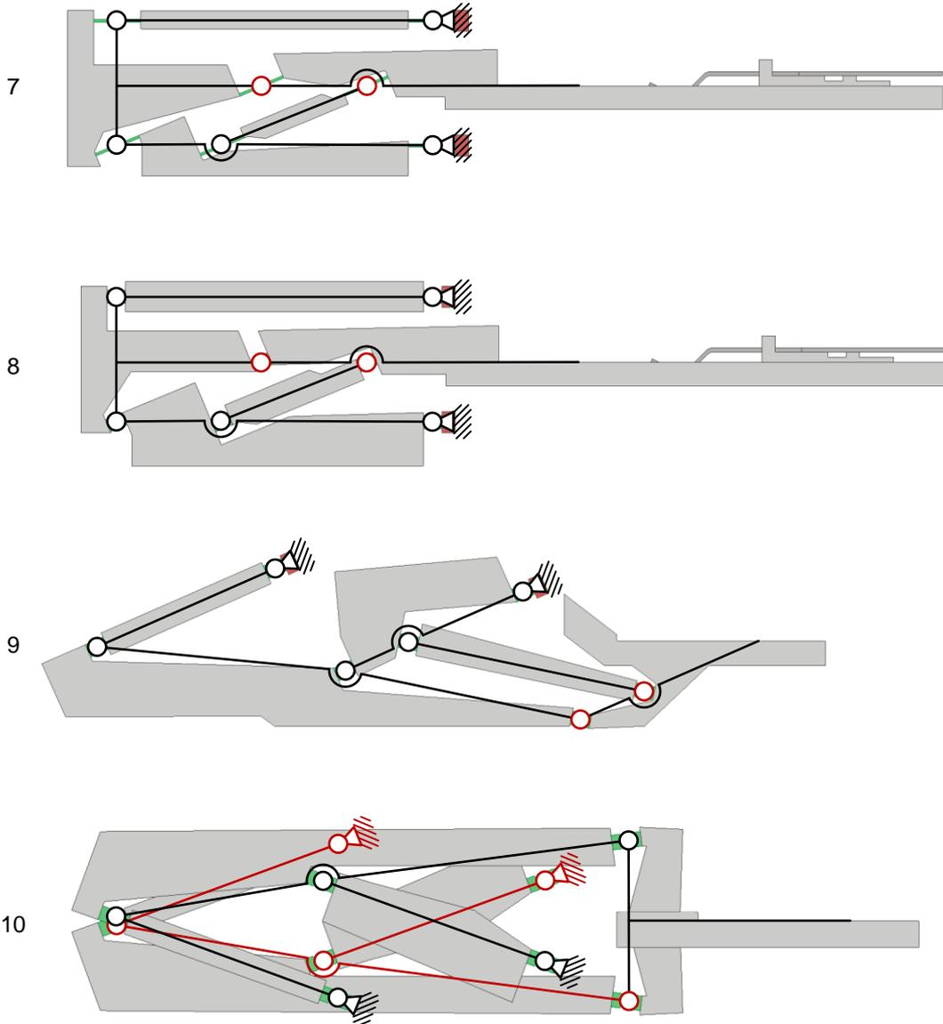
Fig. 13. The rigid body mechanics of concepts 7-10 overlaid on the side view of the concepts.
