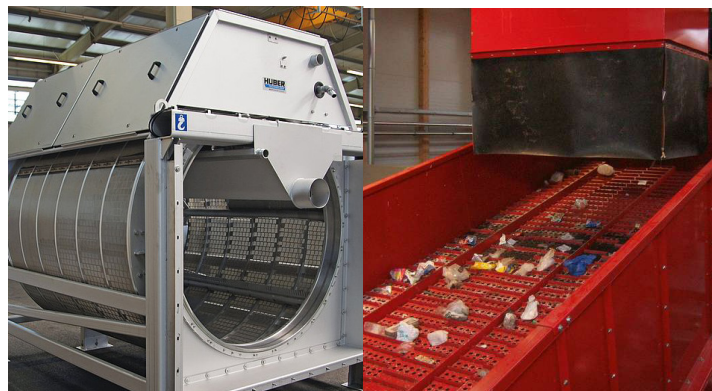
Figure 11 - Rotating Drum Screen
