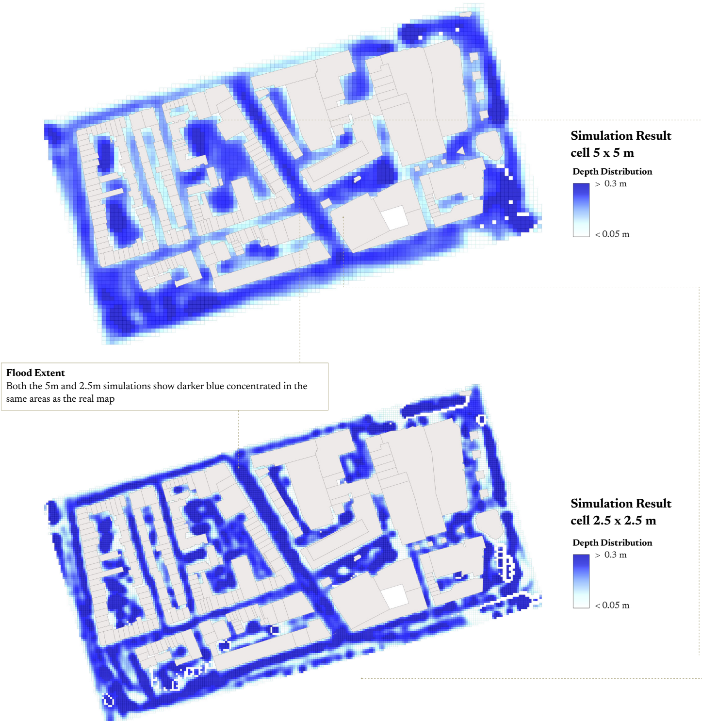
Figure 69. Comparison between simulation result with cell 5 \times 5 m, cell 2.5 \times 2.5 m, and Climate Impact Atlas Map
