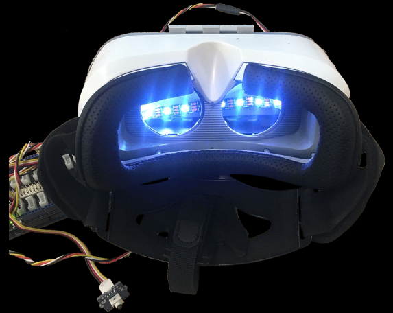
Figure 38: Stimulus hardware setup used in the Flicker protocol.
