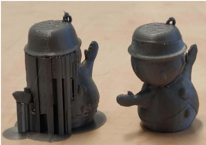
Fig. 1. Snowman models fabricated with an off-the-shelf FDM printer (left) and our multi-directional printing system that adds only one rotational axis to the same printer (right). By allowing material accumulation along different directions in different regions, our system substantially reduces support necessitation.
