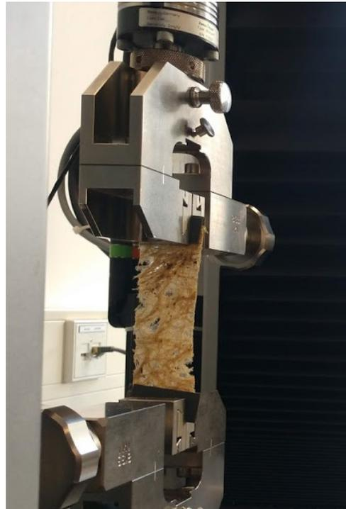
Figure[4.7]: Zwick/Roell Z010 Tensile Tester Figure [4.8]: Test setup with a randomly oriented sample
