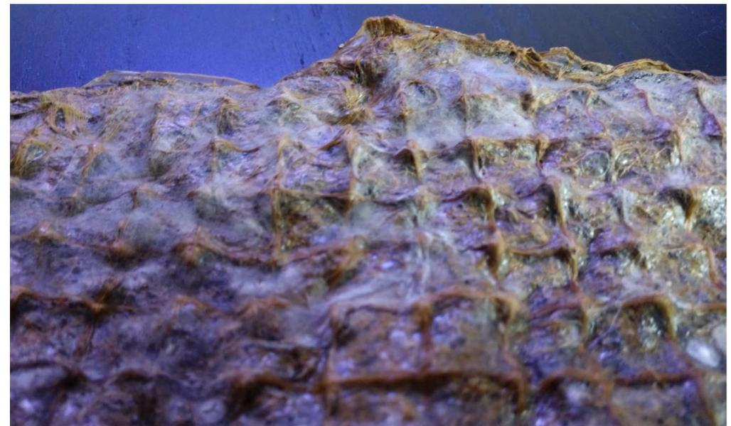
Figure [3.10]; Agar-root composite grown in agar (top) and infused with agar (bottom)
