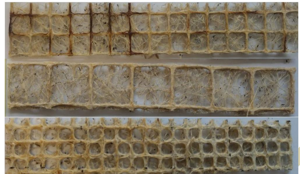
Figure [4.37]: ASTM D5035 samples for (top) 1cm cell, (mid) 2cm cell, and (bottom) 0.5cm cell-sized grids.
