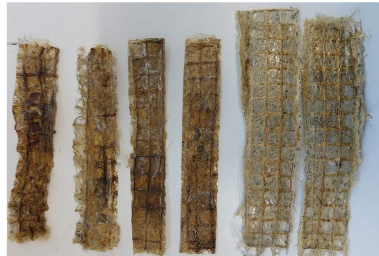
Figure [4.47] ASTM D3039M Samples (Individual)
