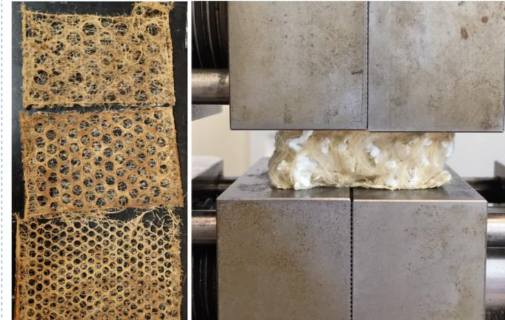
image / figure 1: Compression tests of Interwoven textile with embedded PLA structures
