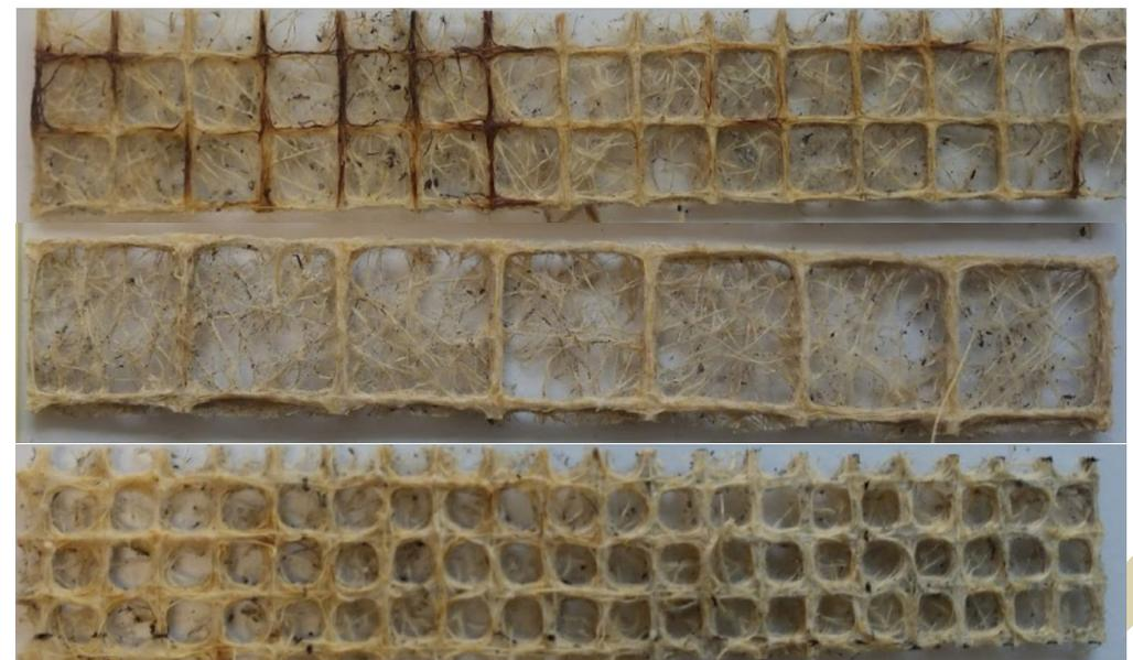
Figure [B.28]: ASTM D5035 samples for (top) 1cm cell, (mid) 2cm cell, and (bottom) 0.5cm cell-sized grids.
