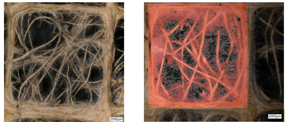
Figure [4.34]: Fiber root density measured on a 1cm cell
