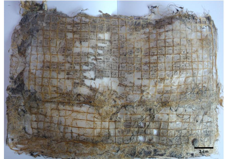
Figure [4.44]: Agar-Root composite sheet (bulk clamped)
