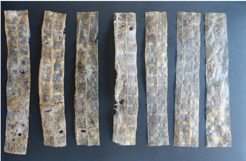
Figure [4.45] :ASTM D3039M samples (bulk)
