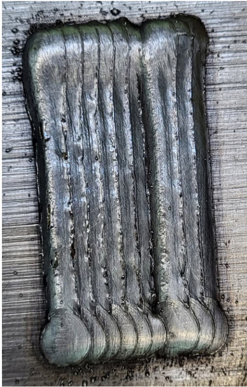
Figure 3.19: 60 % overlap - 1st layer
