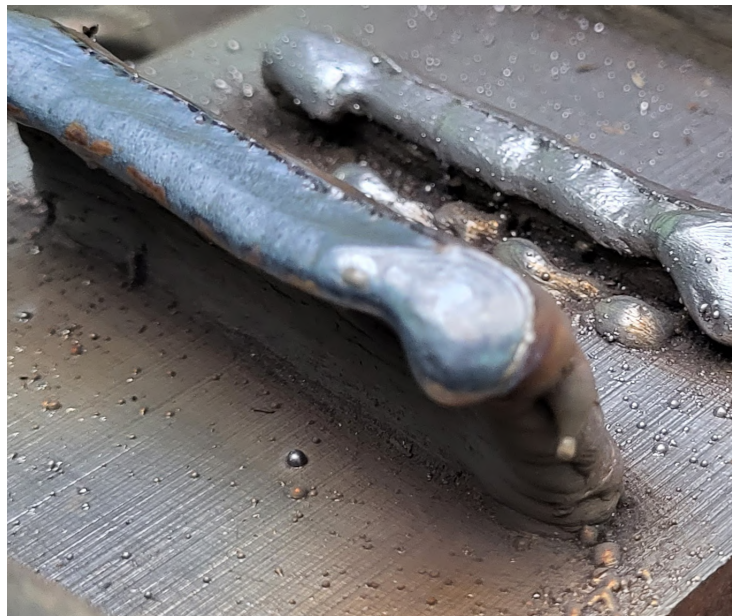
Figure 3.9: Overflow of the weld pool in layer 12
