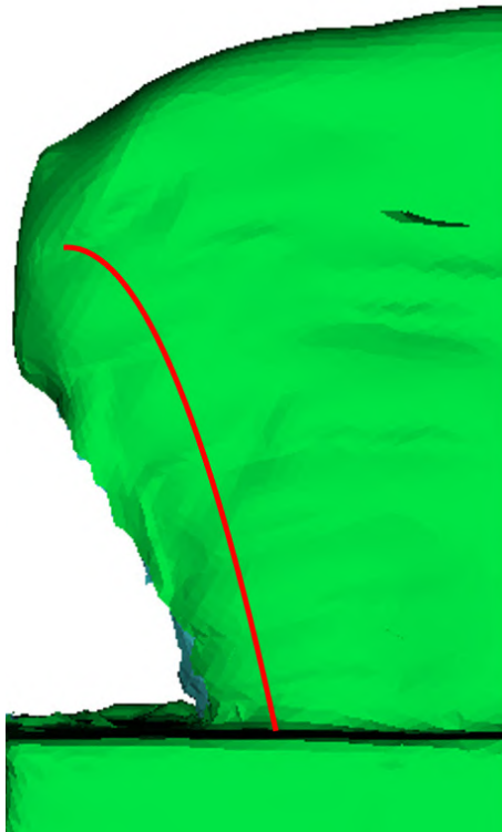
Figure 3.15: Accuracy of the printed overhang
