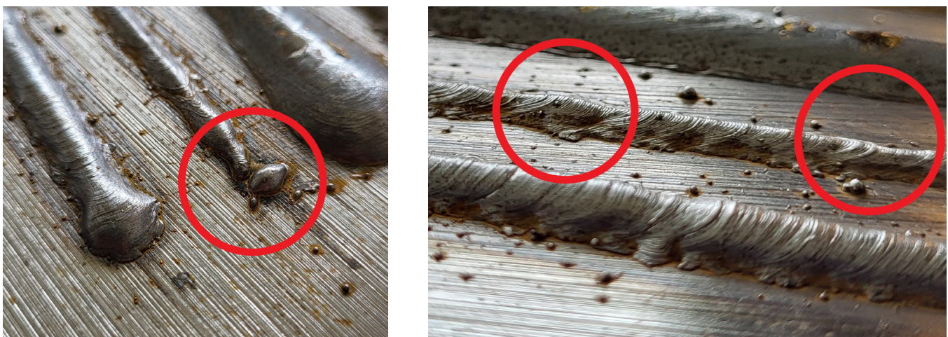
Figure 3.3: Welding defects (waviness, discontinuity, low accuracy at the start and end of the print) in sample 4
