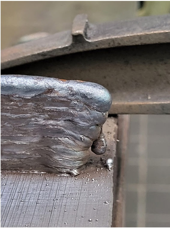
Figure 3.14: Overflow of the weld pool in layer 9
