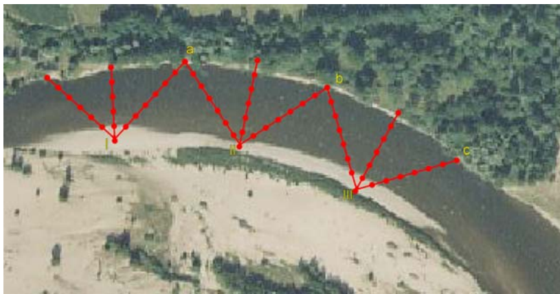
Figure 4-11, Water levelling sections. The levelling instrument is positioned in I, II and III. The dots depict the measured locations. The different levelling sections intersect at a, b and c.
