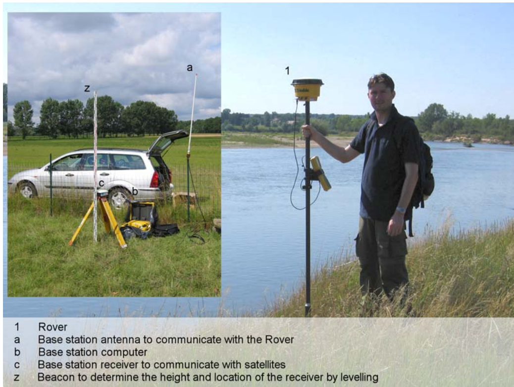
Figure 4-9, Measuring with the RTK-DGPS rover and base station (Baptist, July 2004).
