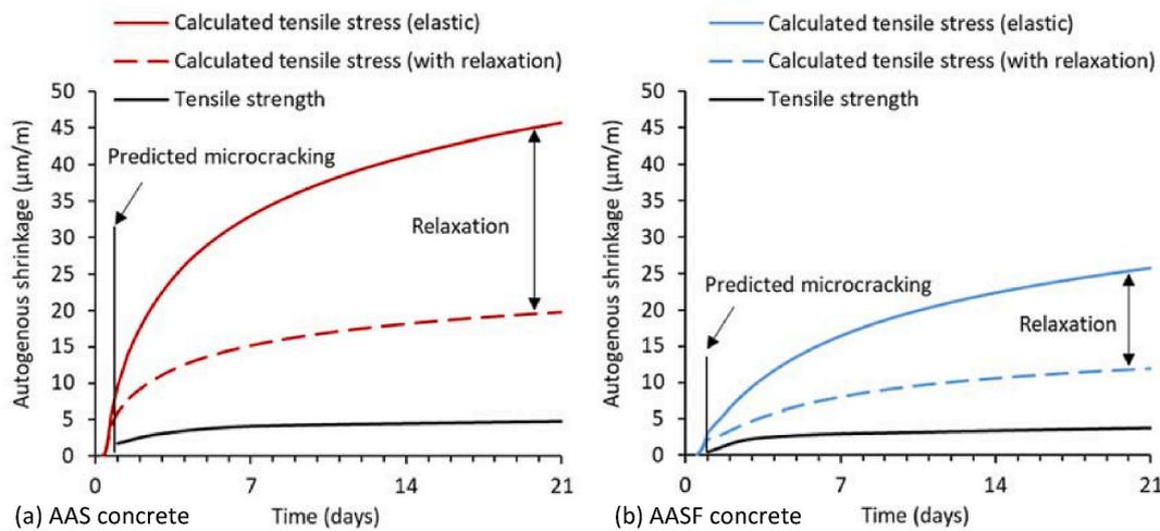
**Fig. 13.** Calculated tangential tensile stress with (dashed lines) and without (solid lines) consideration of relaxation in AAC concrete (a) and AASF concrete (b). The stress is compared with the measured tensile strength of AAC and AASF concrete strength (solid black lines, see Fig. 2 (b)). The calculated tensile stress appears higher than the tensile strength at 1 day of curing, as marked by the arrow.
