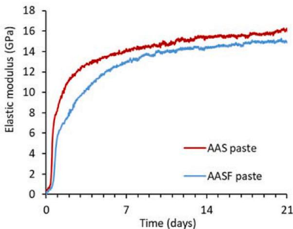
Fig. 4. Measured elastic modulus of alkali-activated paste.
