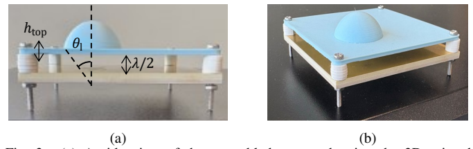
Fig. 3. (a) A side view of the assembled sensor showing the 3D printed dielectric lens with a truncation angle ( \theta_1 ) of 36^\circ and an extension thickness ( h_{\text{top}} ) of 1.92 mm. (b) The assembled sensor placed on \frac{\lambda}{2} (at 26.5 GHz) extensions to create the air cavity between the feed and the lens.
