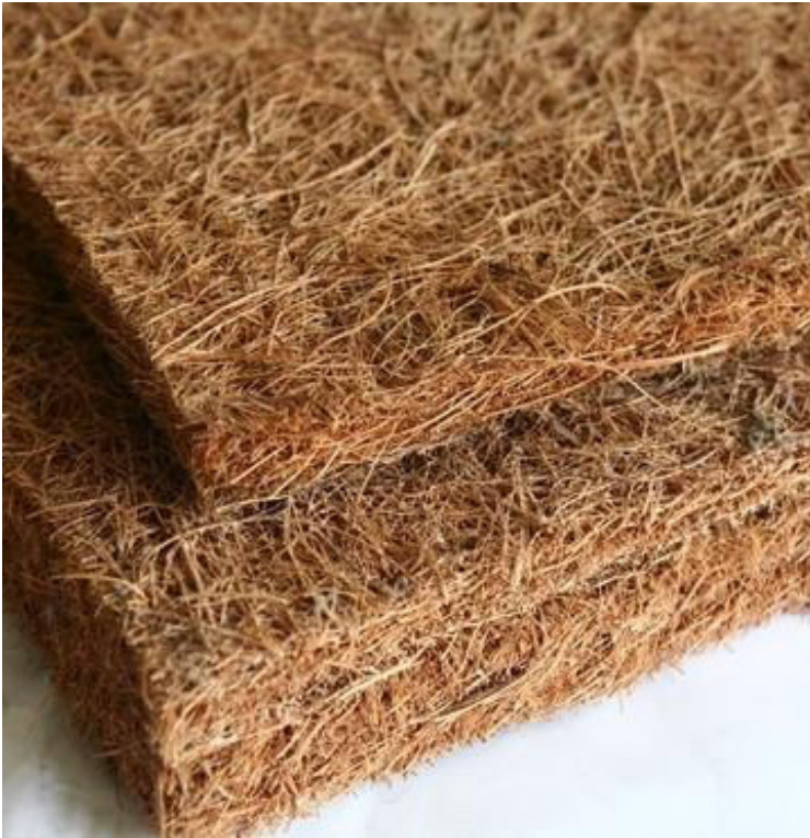
insulation - natural coconut fiber
