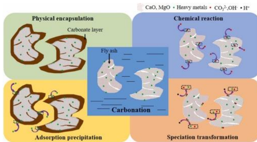
Figure 3.7: Mecahnisms of heavy metal immobilization by carbonation of fly ashes (Yuan et al., 2023).
