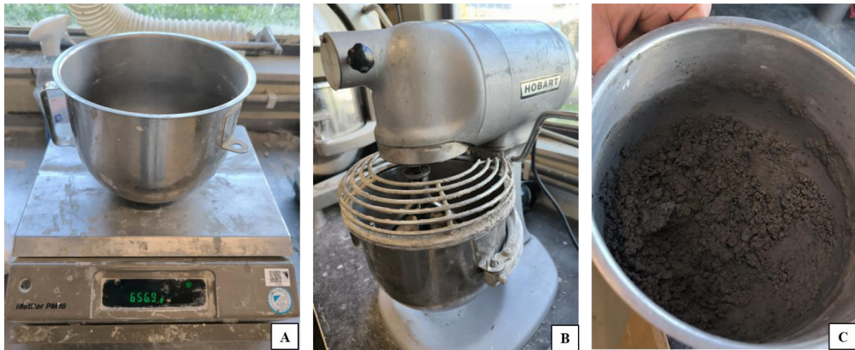
Figure 4.7: (A) Measuring scale for preparation of fly ash-binder-water mixture. (B) Hobart industrial mixing device used for mixing the materials before casting. (C) Ideal earth-moist texture of reference sample after mixing.
