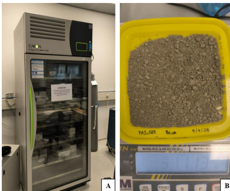
Figure 4.3: (A) Carbonation chamber at fixed temperature of 20°C, pressure of 1 bar, RH of 65% and 1% CO 2 . (B) Sample holder for the fly ashes to ensure maximum contact surface to the environment.
