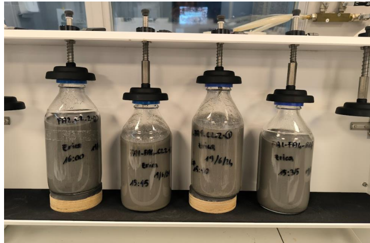
Figure 7.2: Leaching bottles in the end-over-end tumbler after one day of shaking.
