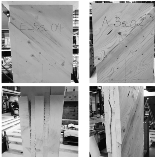
Figure 33 - Specimen failed net-shear (left) and gross-shear (right) (Brandner, Dietsch, et al. 2015)
