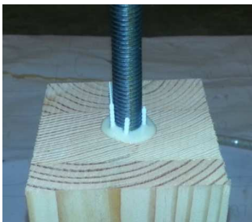
Figure 4 - Glued-in rod in glued-laminated timber (Gonzales, Tannert and Vallee 2016)
