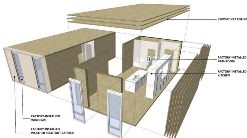
Figure 3 - Modular CLT residential unit (Thompson 2013)
