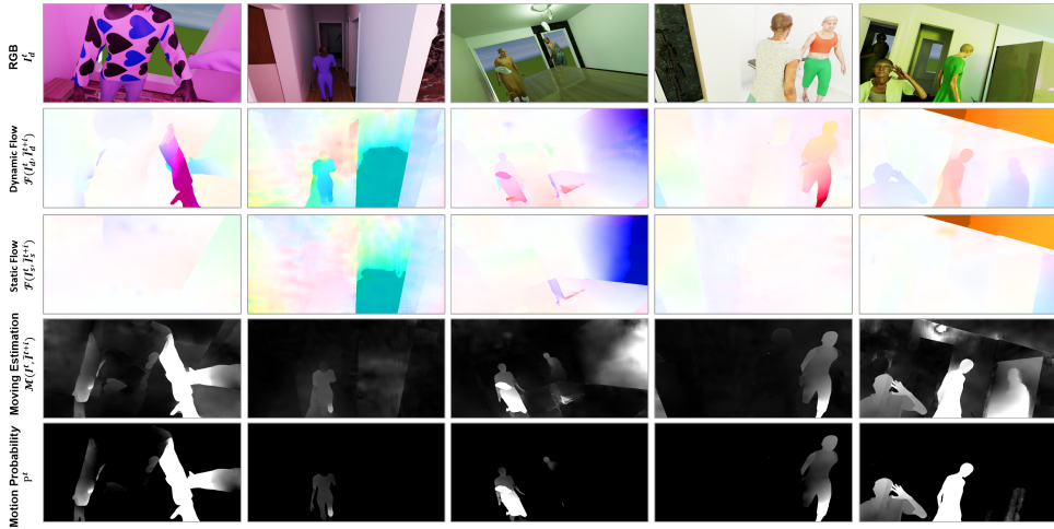
Figure vi: Visualization of the moving estimation and final motion probability. The second line and third line represent the flow estimated on dynamic scenes \mathcal{F}(I_d^t, \tilde{I}_d^{t+1}) and static scenes \mathcal{F}(I_s^t, \tilde{I}_s^{t+1}) respectively, exhibiting similar estimation errors in common static regions. The fourth line demonstrates the moving estimation \mathcal{M}(I^t, \tilde{I}^{t+1}) through flow differencing. The fifth line denotes the blended motion probability P^t by multiplying movable probability p_m^t
