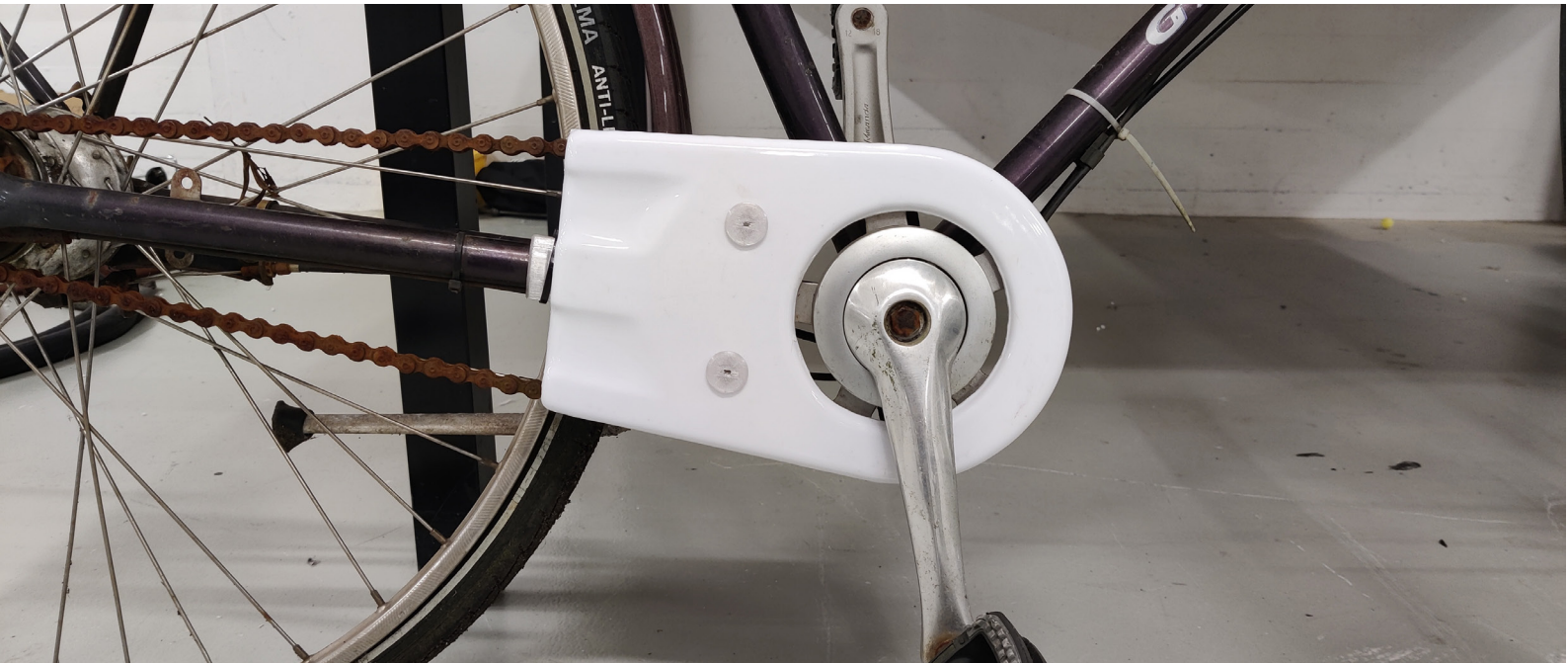
Figure 47: Chain guard prototype installed on a bicycle
