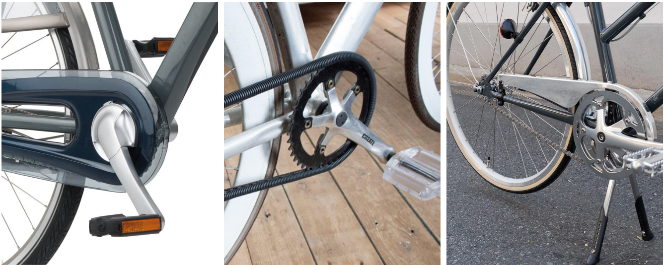
Figure 45: Three categories of chain guards: fully enclosed (Kettingscherm Axa Multi Open), chain runner (De slimme kettingbeschermer), partially enclosed (Tokyobikes - Alloy Chain Guard)
