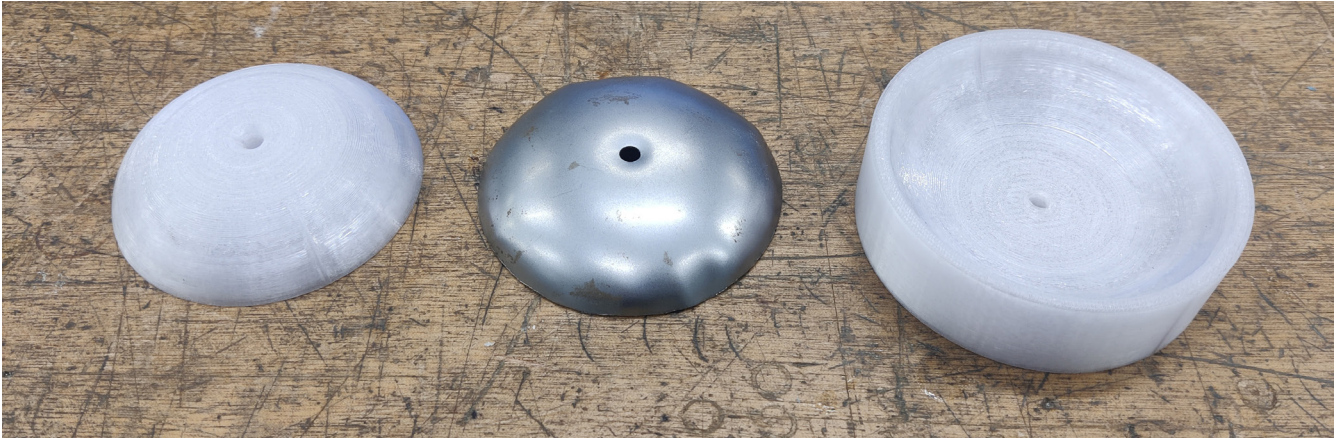
Figure 40: The first prototype - A bell made with 3d printed moulds
