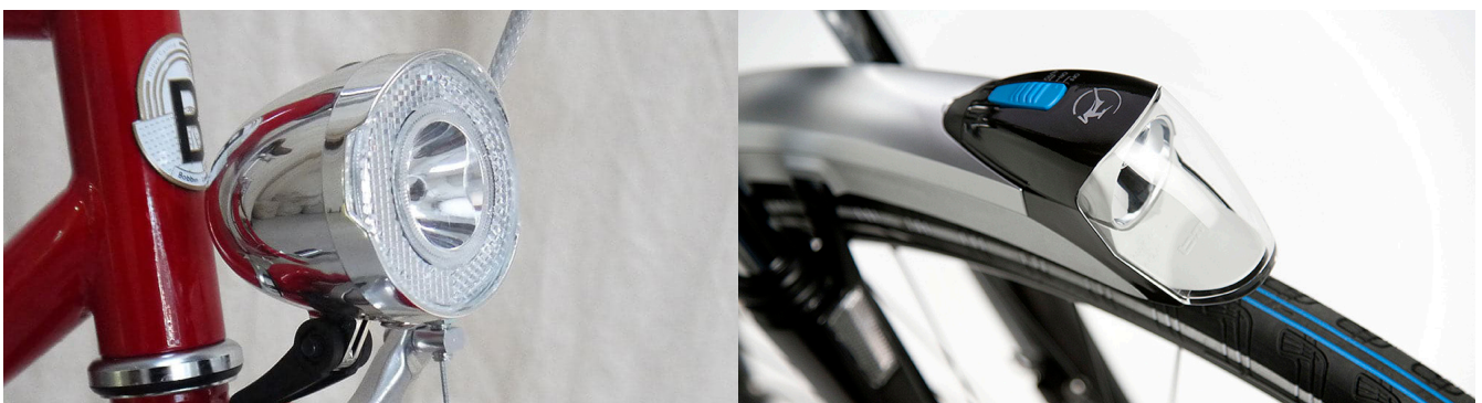
Figure 11: Headlight integration - Classic headlight (Bobbin bikes), modern Gazelle fender vision (Design)
