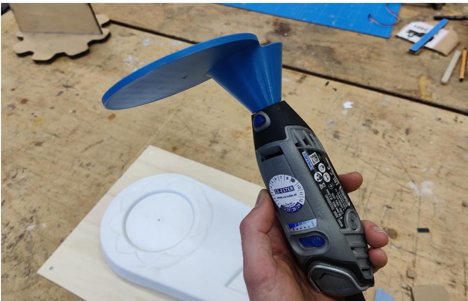
Figure 48: Dremel router jig for cutting a circle
