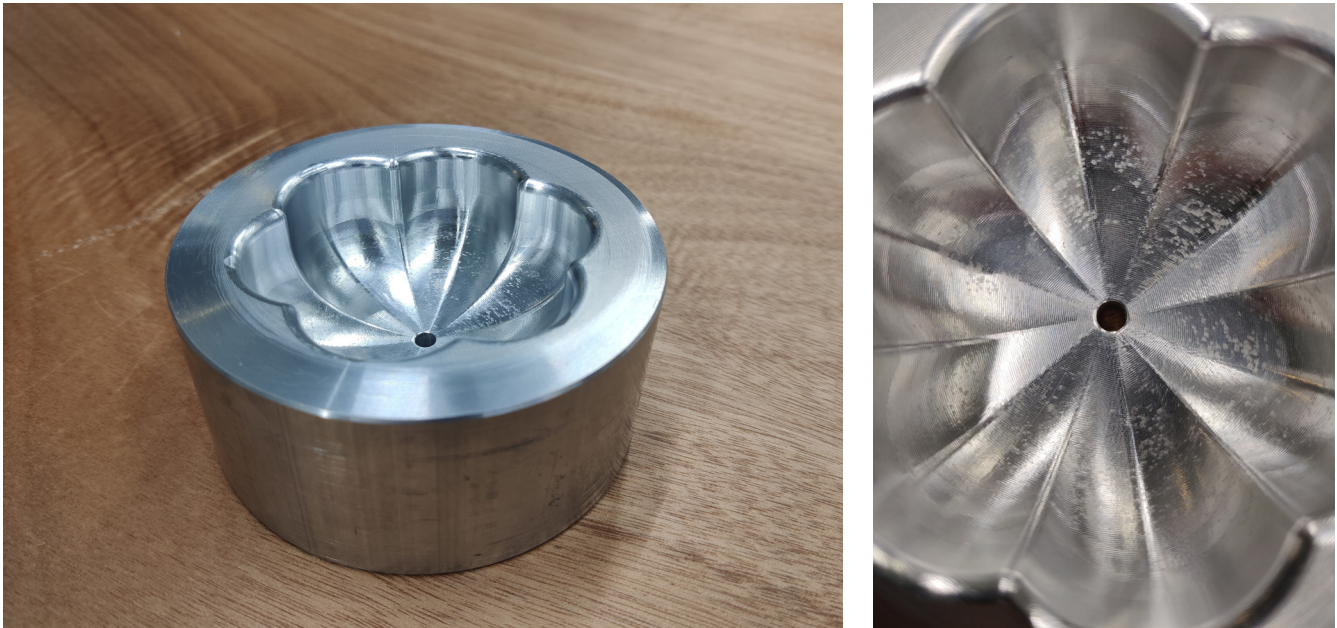
Figure 42: Lower die made from aluminium
