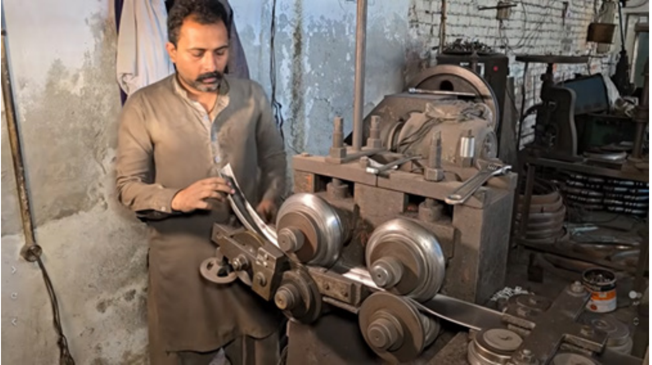
Figure 32: Roller bender in use to make a metal fender (Manufacturing Process Skills, 2025)
