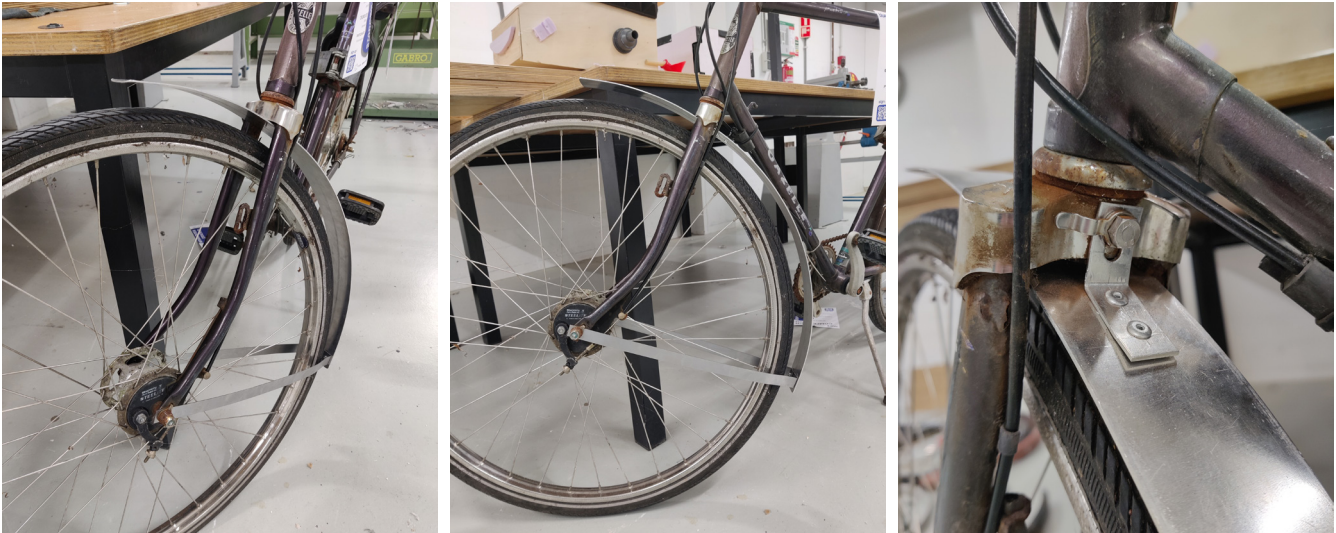
Figure 37: A flat DIY fender made from aluminium
