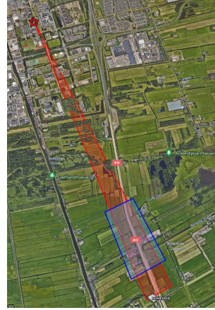
Figure 1.2: Measuring highway vehicles on A13 using PARSAX radar
