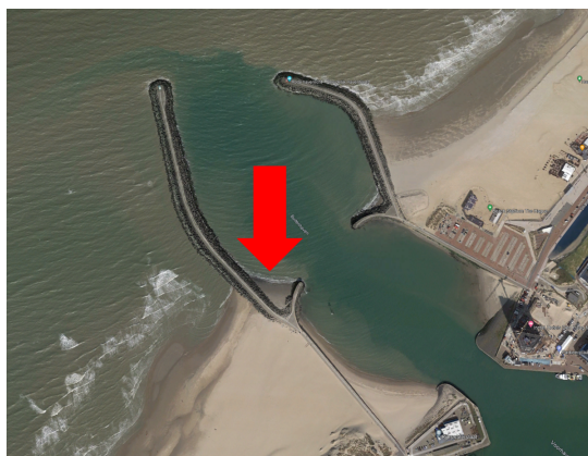
Figure 5.5: The breakwaters of Scheveningen's port. The red arrow shows the buildup of sediment. This means that there is a bypass. Source: Google (2024)
