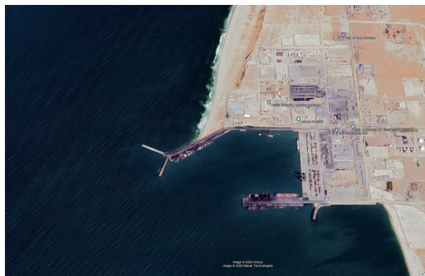
Figure B.11: A satellite image (March 2024) of the breakwater at Nouakchott Harbour. Assumed is no bypassing of sediment. Source: Google (2024).
