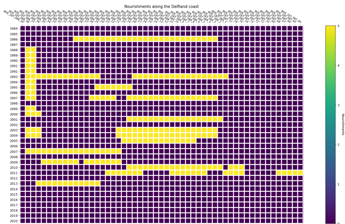
Figure D.3: The nourishment along the Delfland coast on the Satellite-derived Shoreline transects.
