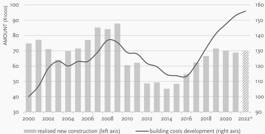
Figure 4.3 Development of annual realised new construction output and indexed construction costs (2000 = 100) in the period 2000 - 2022
