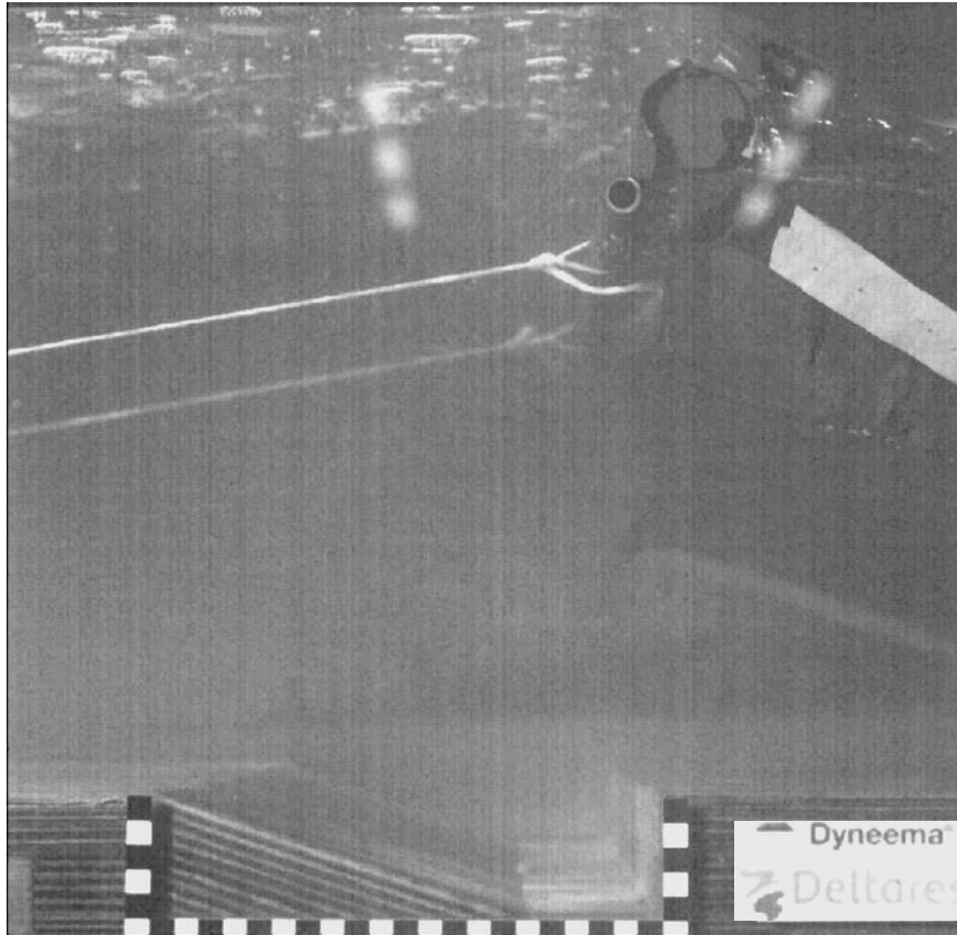
Figure 8. Tsunami of 33 m overflows the barrier (top right), which stays erected.
