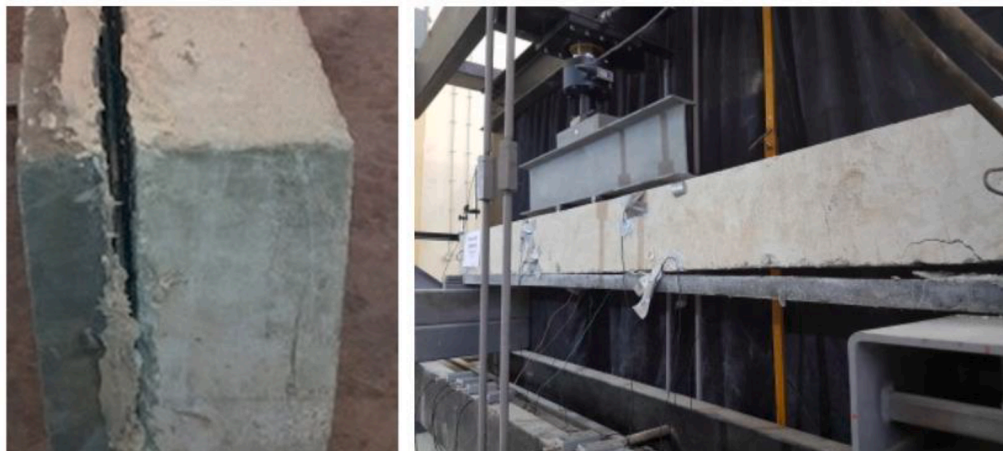
Fig. 24. Debonding at the interface [52,107].
