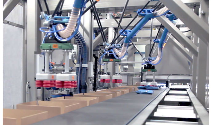
Fig. 1: BluePrint Automation's SPIDER Q series robotic packaging solution [4]. A configuration with three Delta robots with rotational end-effectors and vacuum grippers is demonstrated, picking up pre-packaged food products and placing them into secondary containers.
