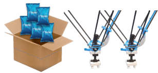
Fig. 3: A complete schedule contains two Delta robots, one box and five products divided into two layers. The task scheduler assigns the layers of a box to the Delta robots with the available products on the conveyor belt, aiming to maximize the number of packed products per minute. Each layer is placed in a single operation by a Delta robot.
