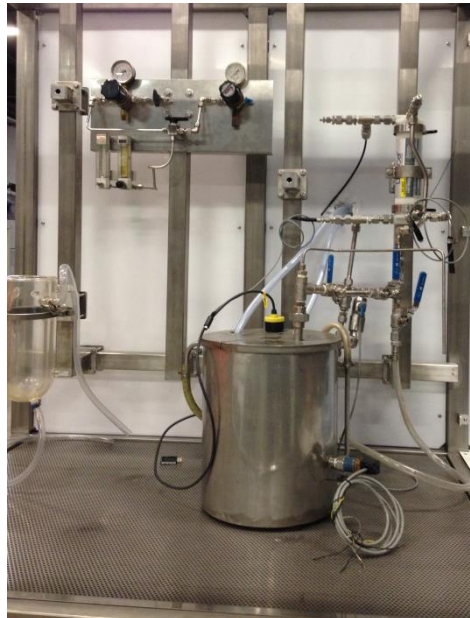
Figure 3.6: Buffer vessel with membrane unit
