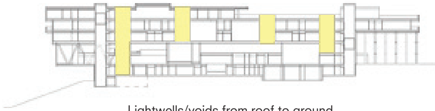
Lightwells/voids from roof to ground
