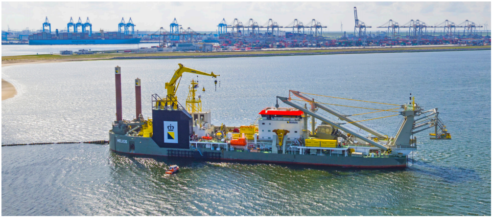
Figure 1.3: The self-propelled cutter suction dredger "Helios" owned by Royal Boskalis Westminster N.V. Source: Boskalis (2017)
