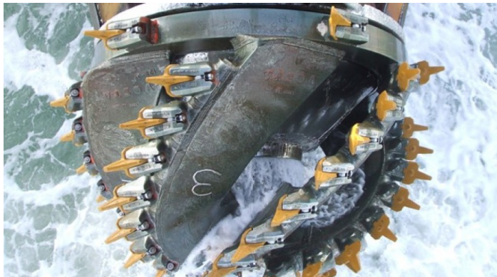
Figure 1.4: The T-series cutter head installed with the third generation cutter teeth manufactured by VOSTA LMG. Source: VOSTA LMG (2020)
