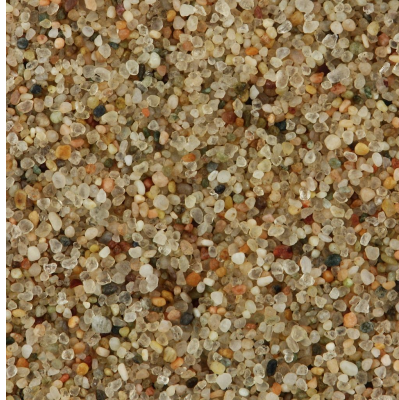
Figure 3.4: Rounded and fine-grained eolian sand sample from the Gobi Desert (near Dalanzadgad in Mongolia). The width of the view is 10 mm (Sepp, 2011)
