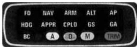
Fig. 3.8: A Mode Annunciator Panel (MAP) From A Bendix / King KFC-200 AFCS (KA-285).
