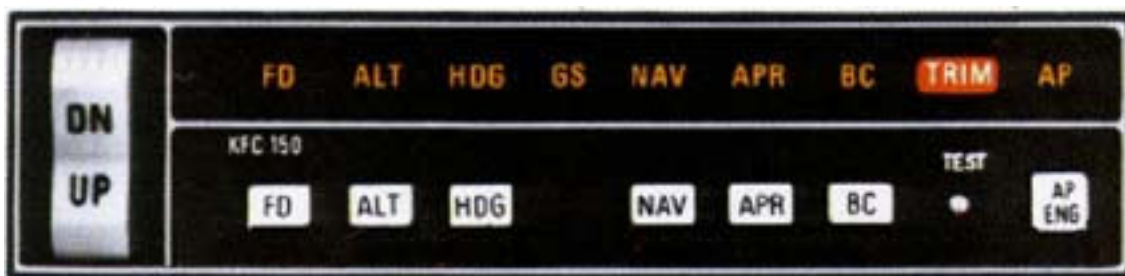
Fig. 3.6: A Mode Control Panel (MCP) From A Bendix / King KFC-150 AFCS (KC-192).
