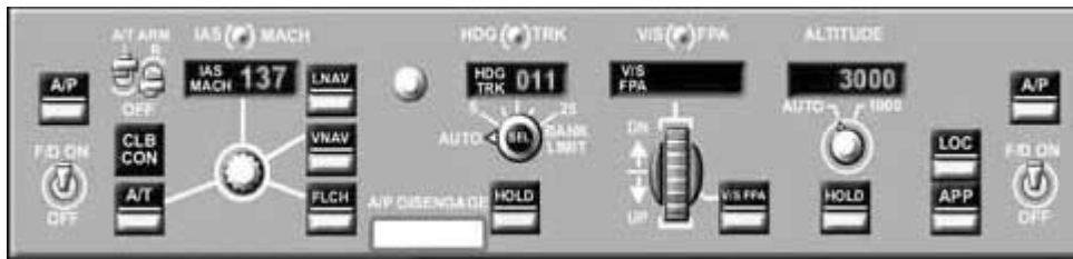
Fig. 3.7: A Rockwell / Collins Mode Control Panel (MCP) Used In A Boeing 777.
