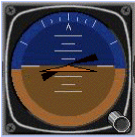
Fig. 3.3: A 'Inverted-V' Type Flight Director.
