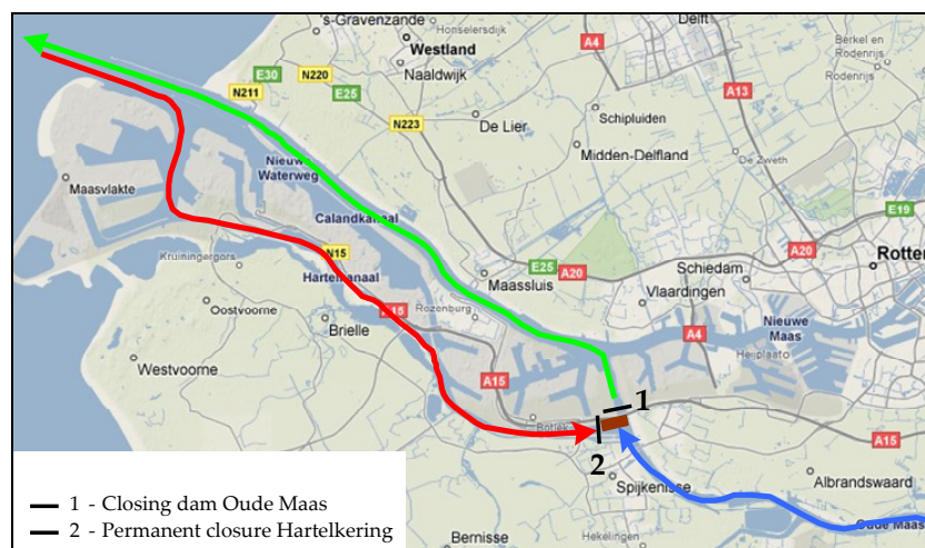
Figure 3: Overview of the different flows for a power plant in the Botlek area. Blue represents fresh, red represents salt, and green corresponds to the brackish flow
