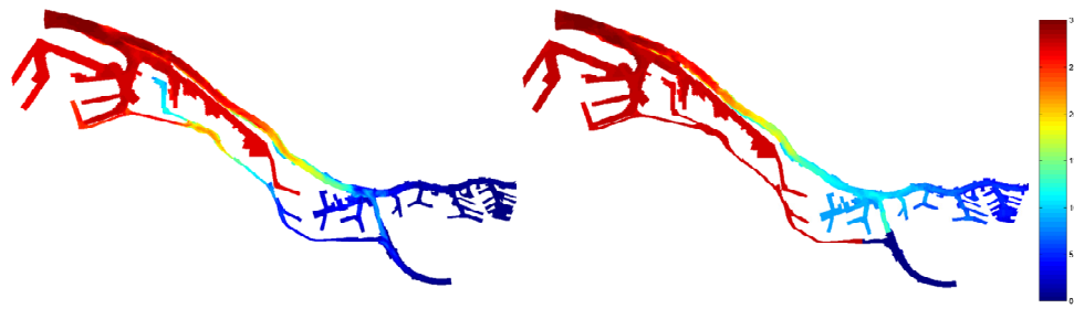
Figure 4: Overview of the changing salt concentrations in the Delta area due to the implementation of a power plant (blue=0g/l, red=30g/l)
