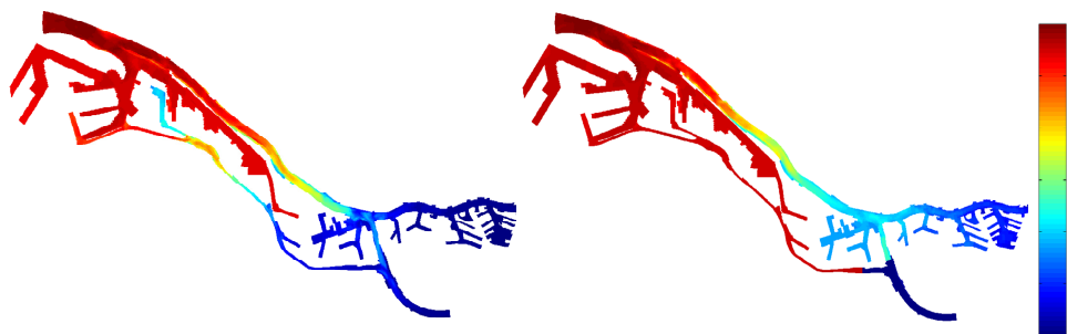
Figure 9.1: Overview of the changing salt concentrations in the Delta area due to the implementation of a power plant (blue=0g/l, red=30g/l)
