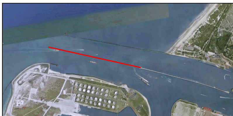
Figure 8.6: Schematic representation of a lengthening of the breakwater between the Calandkanaal and Nieuwe Waterweg, at Hoek van Holland
