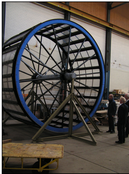
Figure 3.3: Drum for usage in the prefiltration installations
