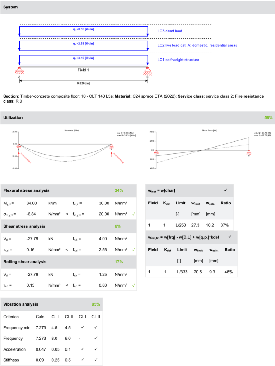
Figure C.10: Summary of static structural verifications for CLT-concrete composite floors, span 6.0m
