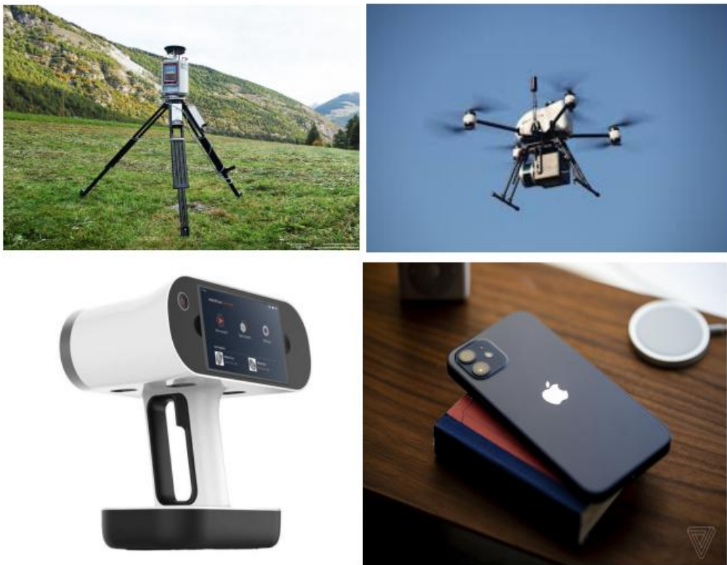
Figure 1.1. Upper left: TLS; upper right: ALS; lower left: hand-held TLS; lower right: iPhone 12
