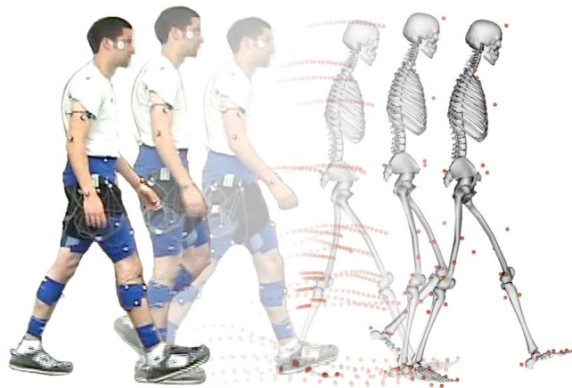
Figure 6: Inverse Kinematics Tool Overview. Experimental markers are matched to model markers for each frame in the captured motion adjusting joint angles, minimizing the overall error between experimental and virtual markers.
