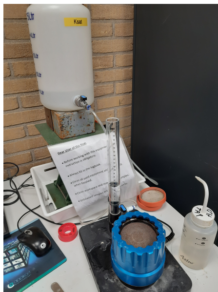
Figure 3.9: KSat device setup during measurement
