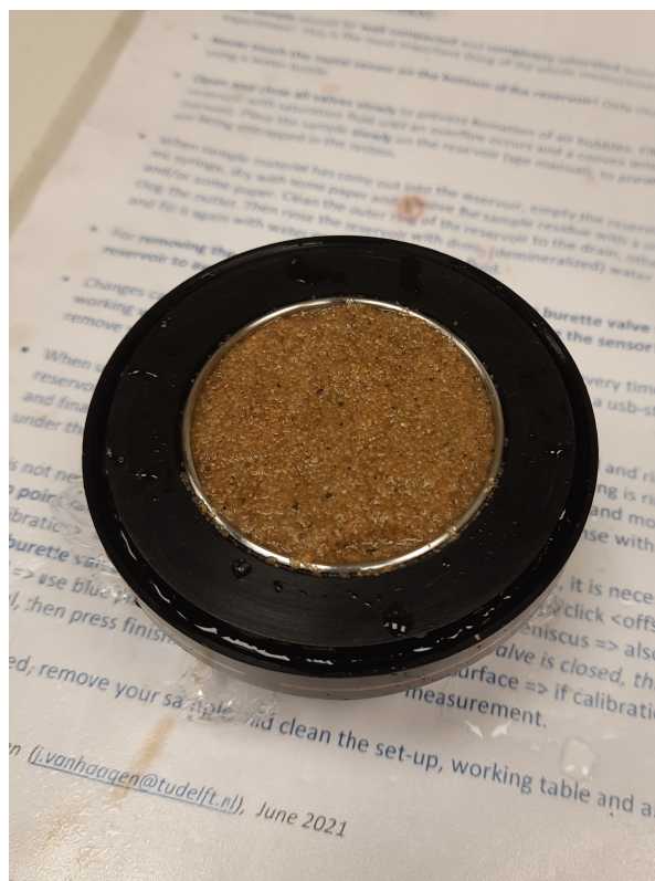
Figure A.6: A saturated sand sample ring in the adapter for the KSat device
