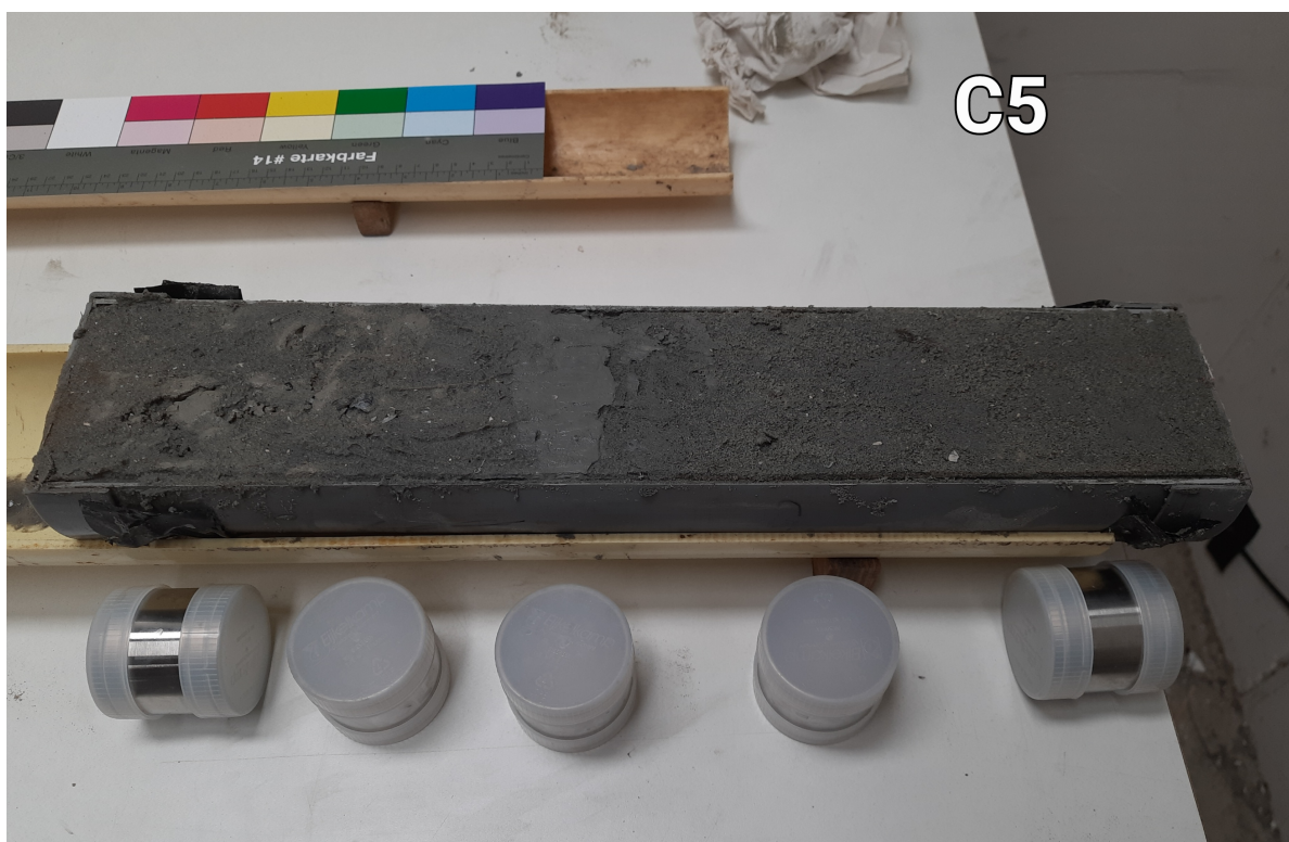
Figure A.4: DAPGEO-02-C5 before plug sampling with the sample rings positioned at planned sampling location and orientation
