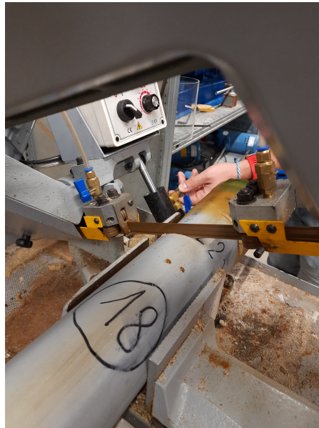
Figure 3.5: Sawing off the top of a sediment core along the marking
