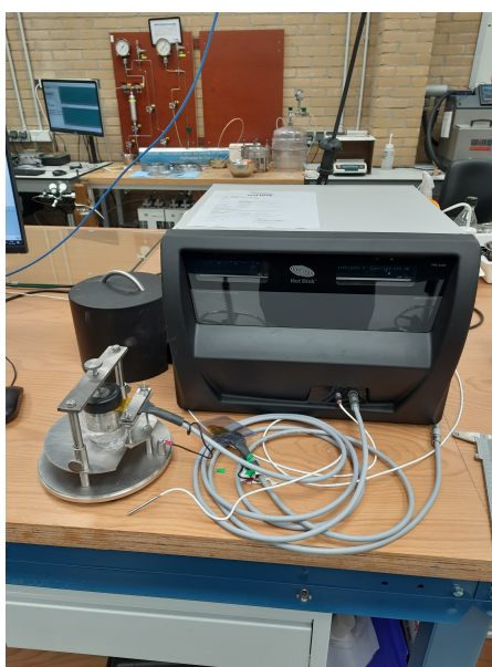
Figure 3.8: Hot disk device setup showing plug screwed in place
