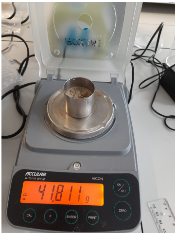
Figure 3.10: RD-05-P1 sample weighing for pycnometer measurement
