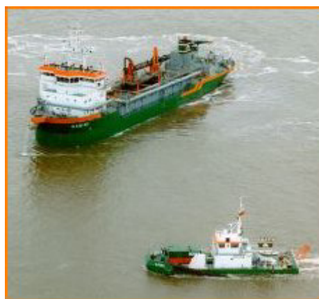
Figure 1: A traditional hopper dredge and a WIS dredger
