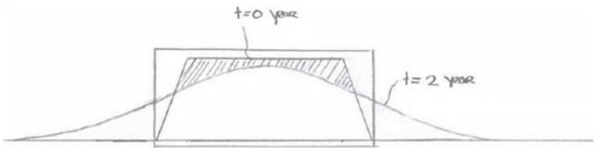
Figure 1.3 – Rectangular 'control element' for which the eroded volumes can be calculated in each year
