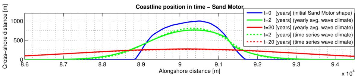
Figure 3.9 – Coastline position of the Sand Motor implemented in UNIBEST-CL+
