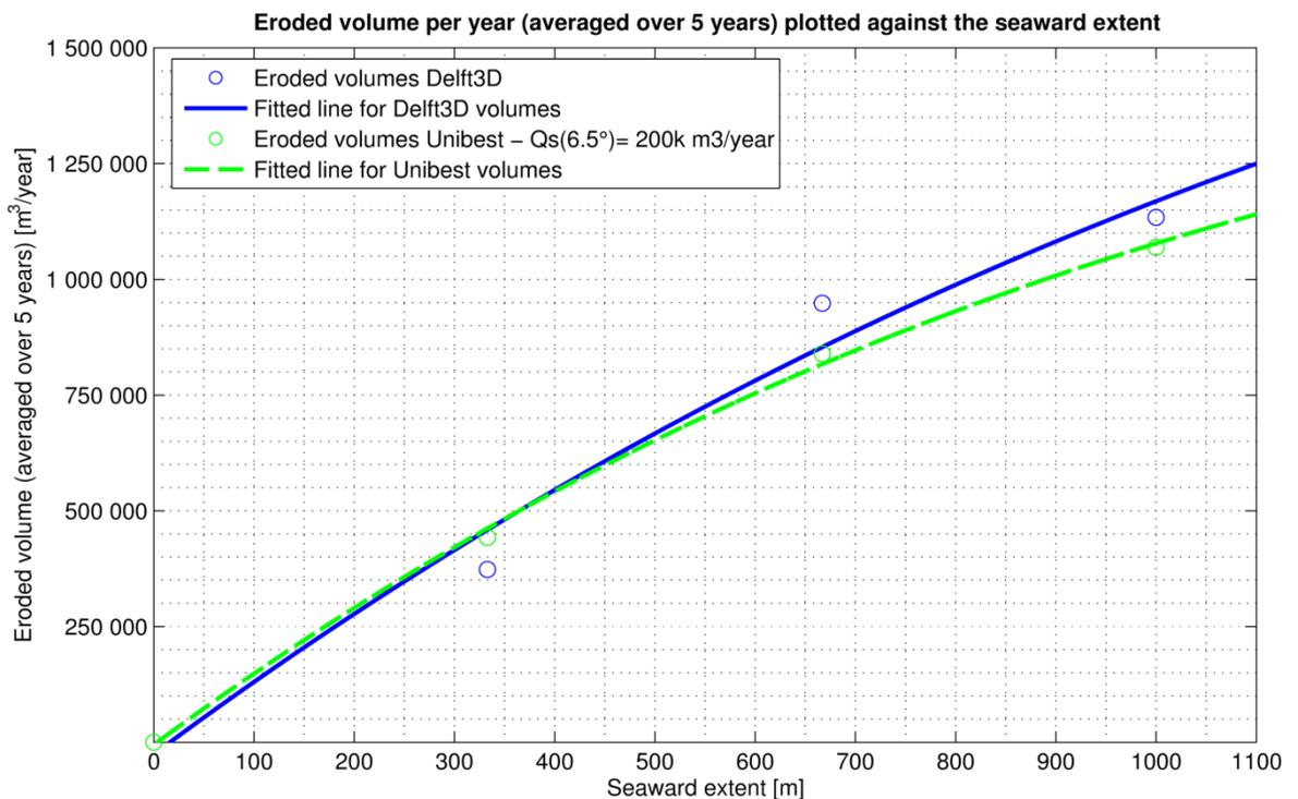
Figure 5.10 – Eroded volume per year (averaged over 5 years) plotted against the seaward extent – D3D & Unibest
