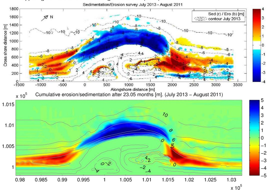
Figure 3.19 – Cumulative erosion/sedimentation: measured (upper) and modelled (lower) after 23 months. Upper figure from Shore Monitoring & Research (2013)
