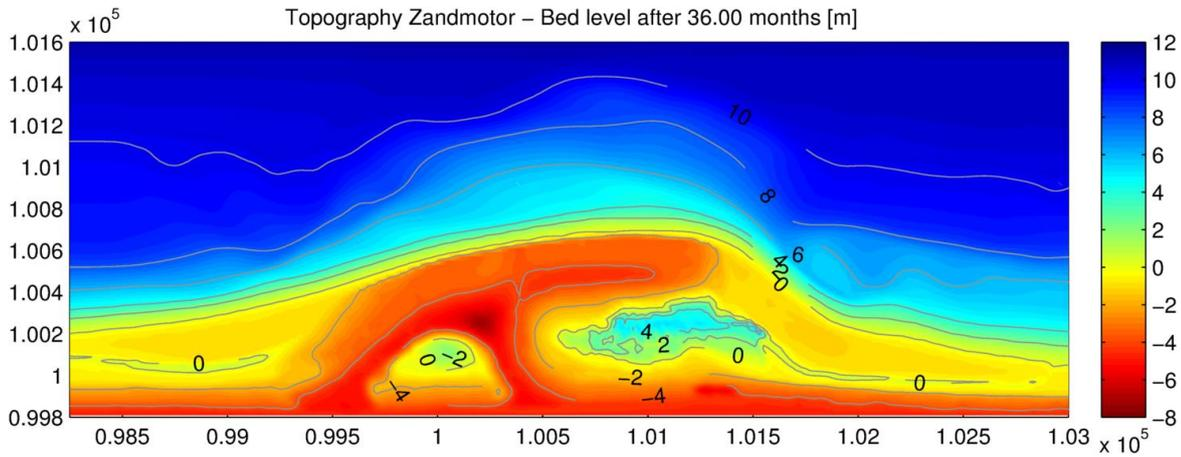
Figure C.1 – Roller model –  $D_h = 0.25 \text{ m}^2/\text{s}$ : Topography Sand Motor after 36 months
