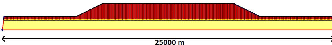
Figure 3.2 – Top view of the biggest nourishment implemented in the UNIBEST-CL+ model
