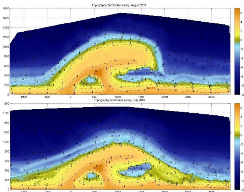
Figure 2.2 – Survey 1: Bathymetry Sand Motor August 2011 (upper) & Survey 18: Bathymetry Sand Motor July 2013 (lower). (Shore Monitoring & Research, 2013)
