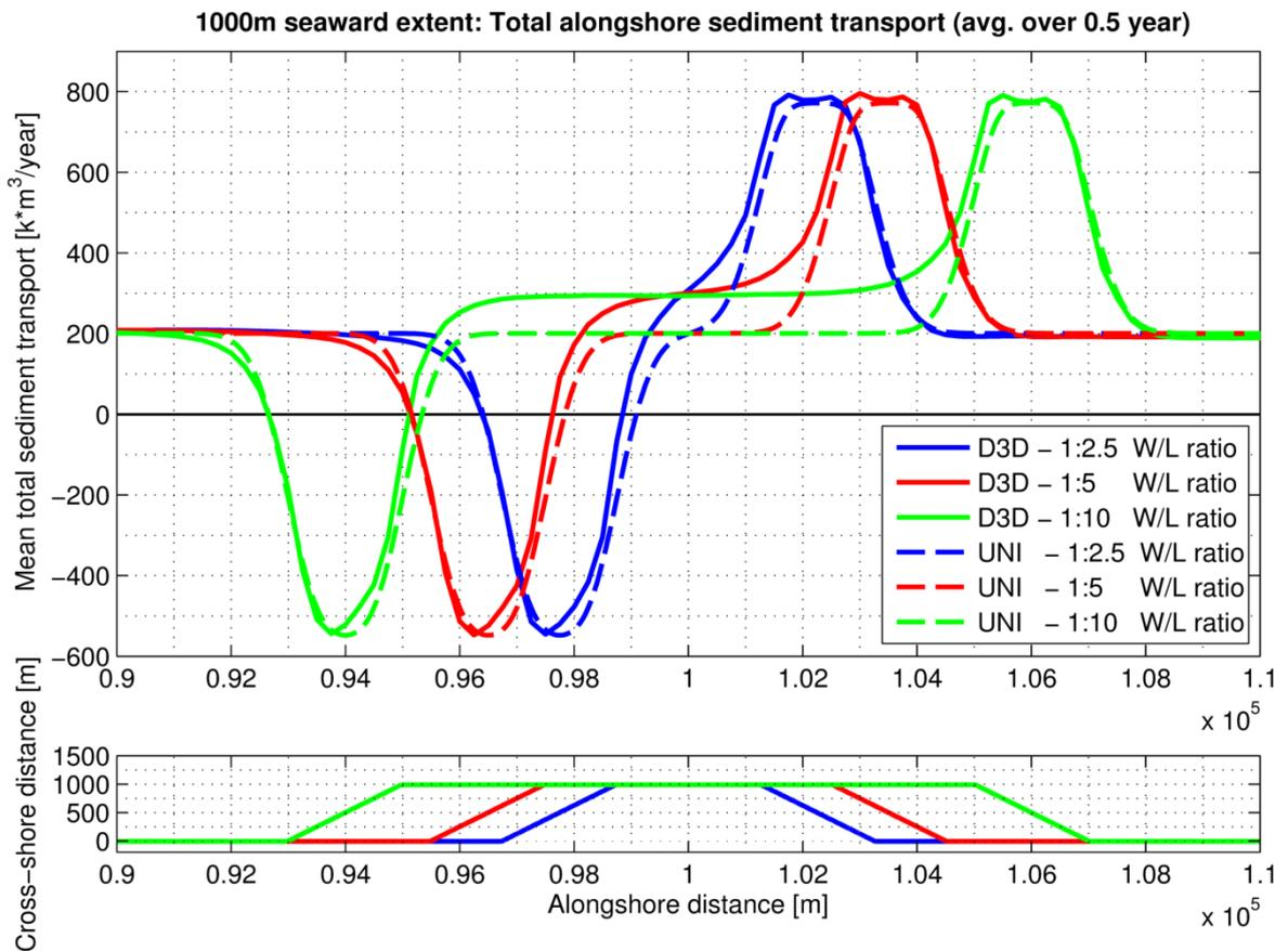
Figure 5.5 – Net alongshore sediment transport vs. alongshore distance for the 1000m seaward extent nourishments
