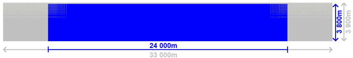
Figure 3.10 – Top view and dimensions of flow grid (blue) and wave grid (grey)
