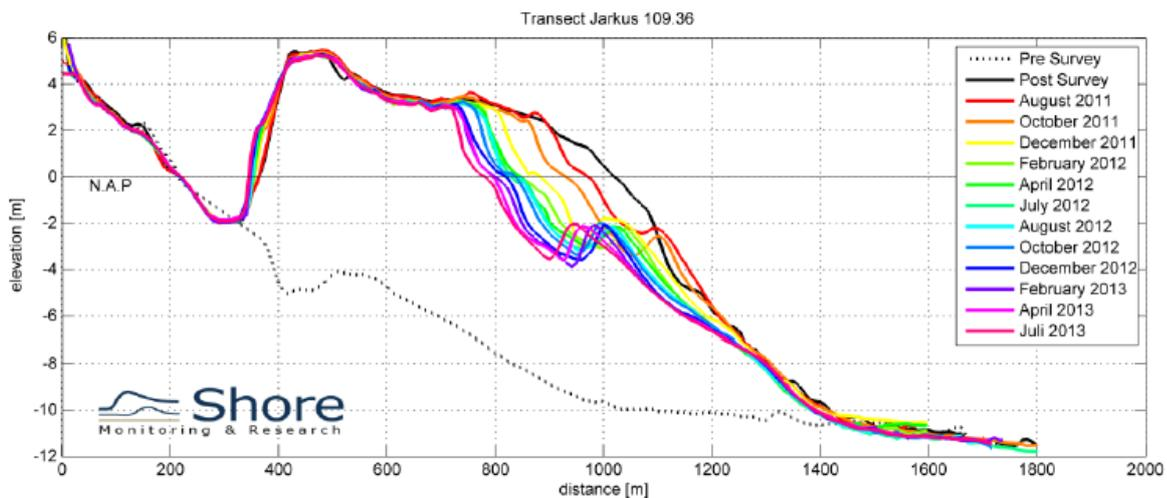
Figure D.2 – Cross-shore profiles for ‘Jarkusraai’ 109.36 located just left at the centre of the Sand Motor (Shore Monitoring & Research)
