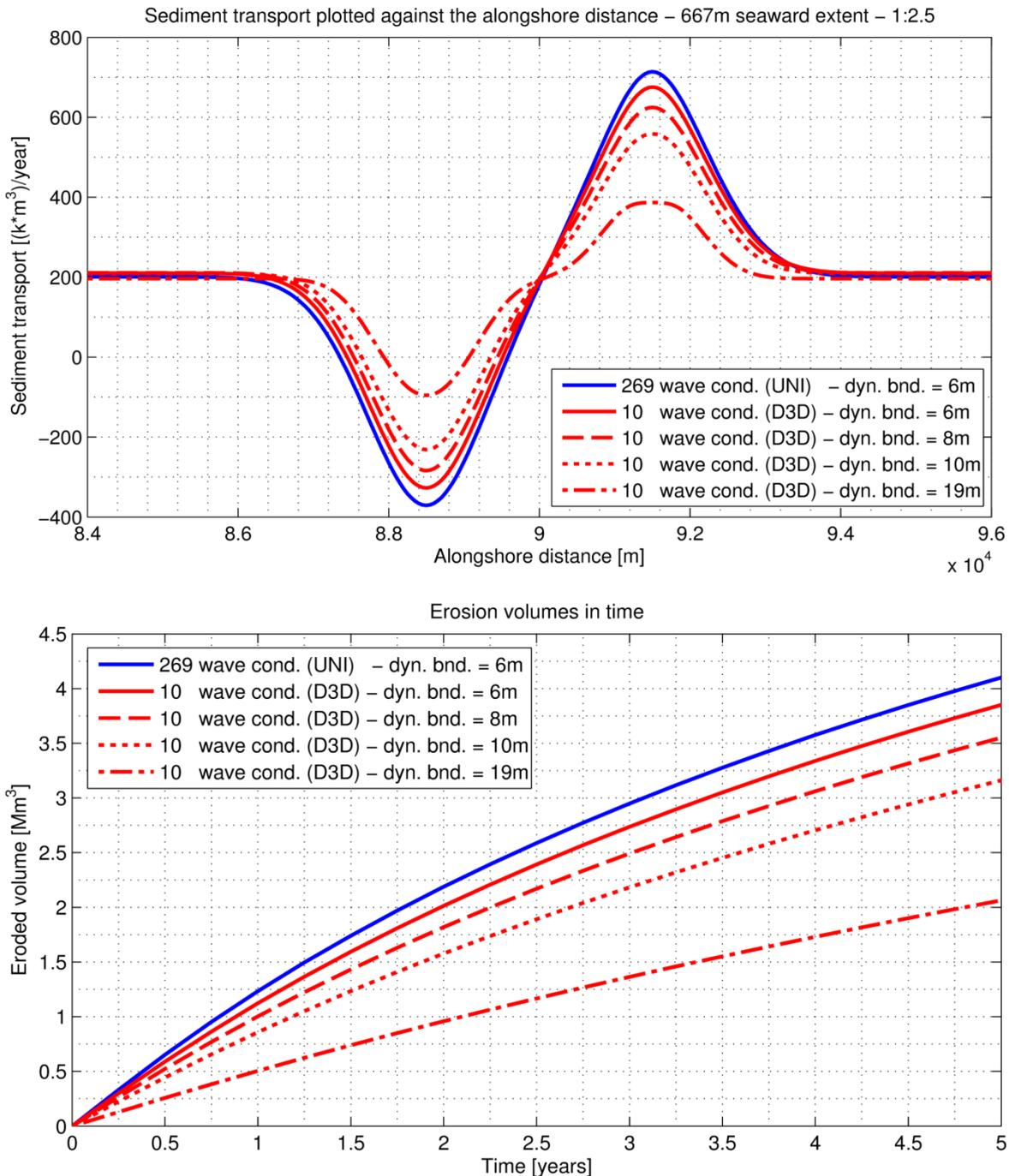
Figure 4.10 – Alongshore sediment transport at  $t=1$  year (upper figure) and eroded volume in time (lower figure)
