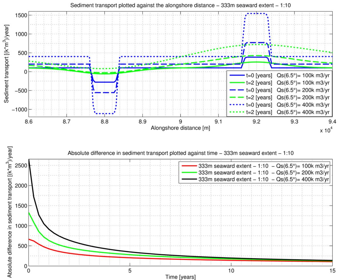
Figure F.4 – Sediment transport in alongshore direction (upper) and in time (lower) for the 333m 1:10 nourishment
