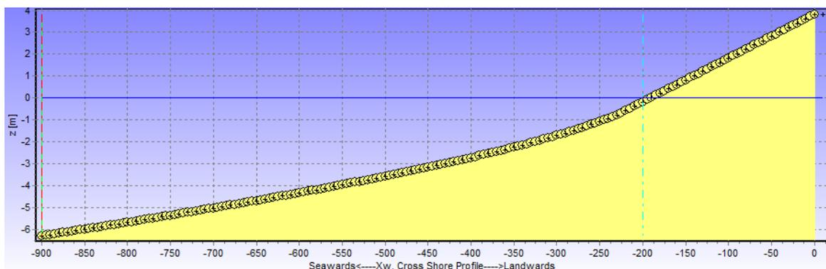
Figure 3.5 – Cross-shore profile which is used for computing the ray file
