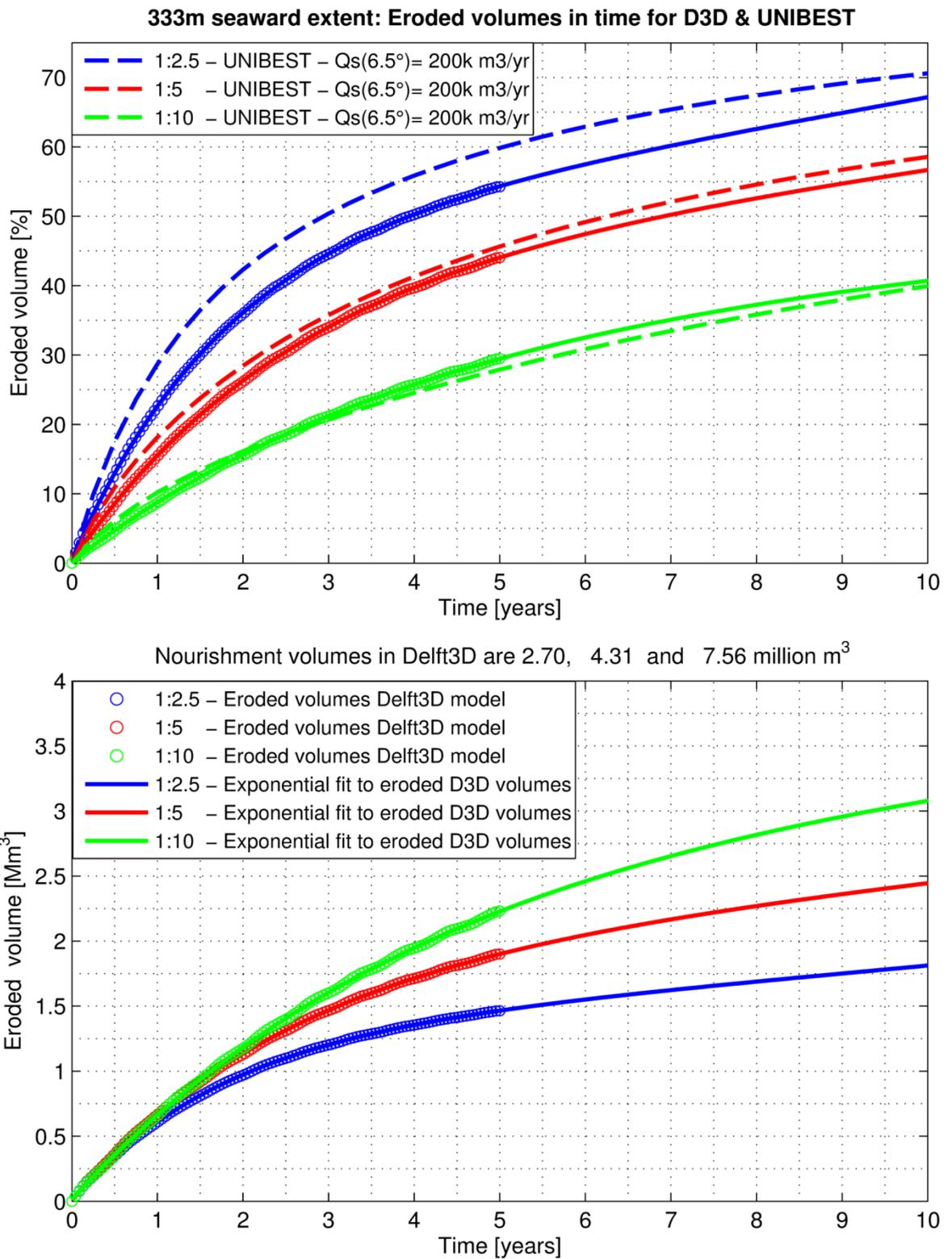
Figure 5.2 – Eroded volumes in time for 333m seaward extent – D3D & UNIBEST
