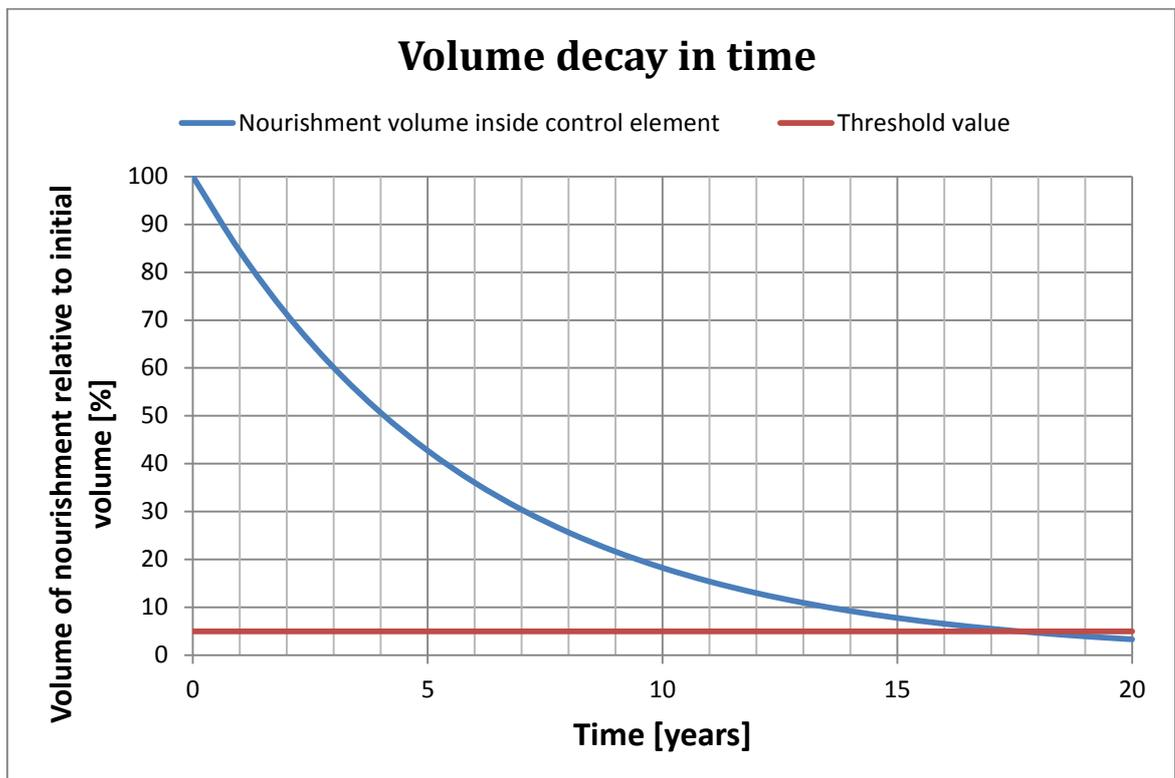
Figure 1.6 – The lifespan is defined as the time it takes for the volume to drop below a certain threshold value
