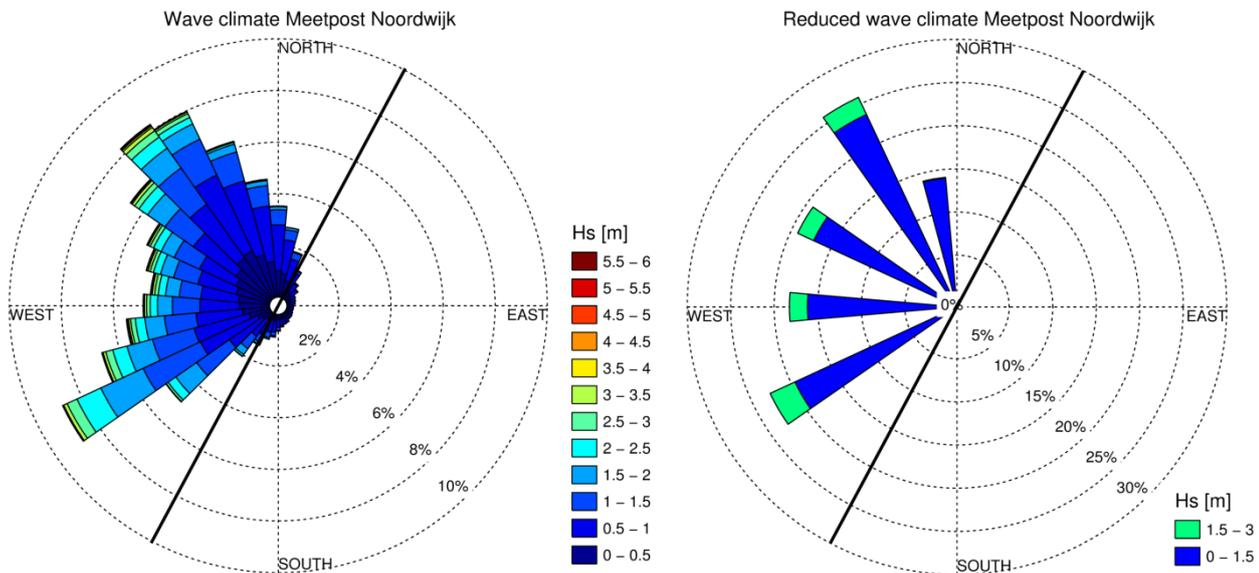
Figure 3.13 – Wave rose of the full wave climate (left) and reduced wave climate (right) at Meetpost Noordwijk
