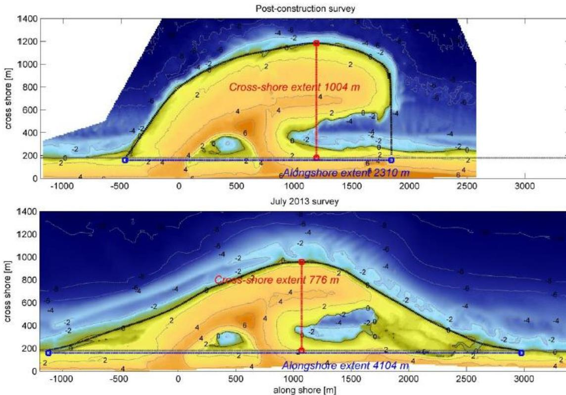
Figure 2.4 – Contour lines of the Sand Motor: post-construction (upper figure) and after two years (lower figure). (Shore Monitoring & Research, 2013)
