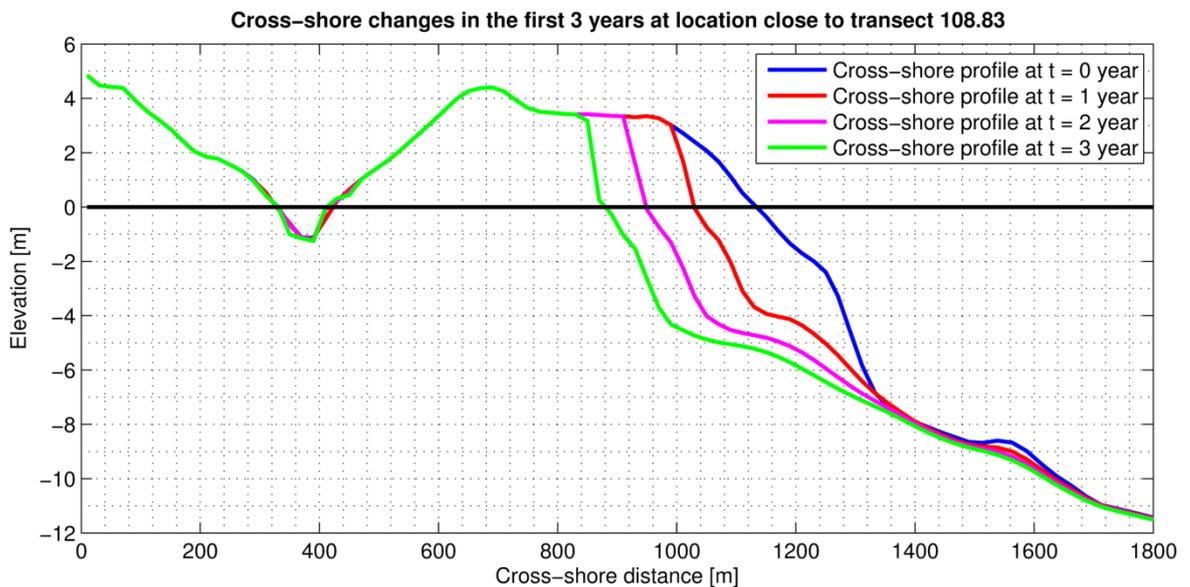
Figure D.4 – Cross-shore profiles for the Sand Motor model in Delft3D for the first three years
