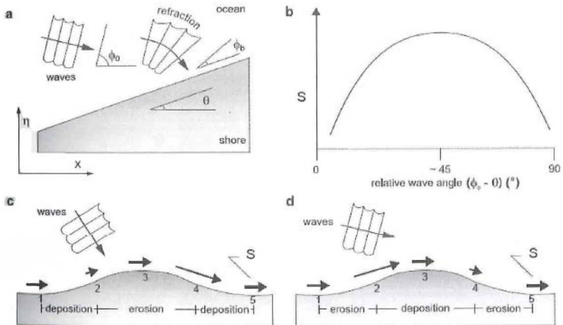
Figure 2.1 – Response of a perturbation in the shoreline to low-angle waves and high-angle waves
