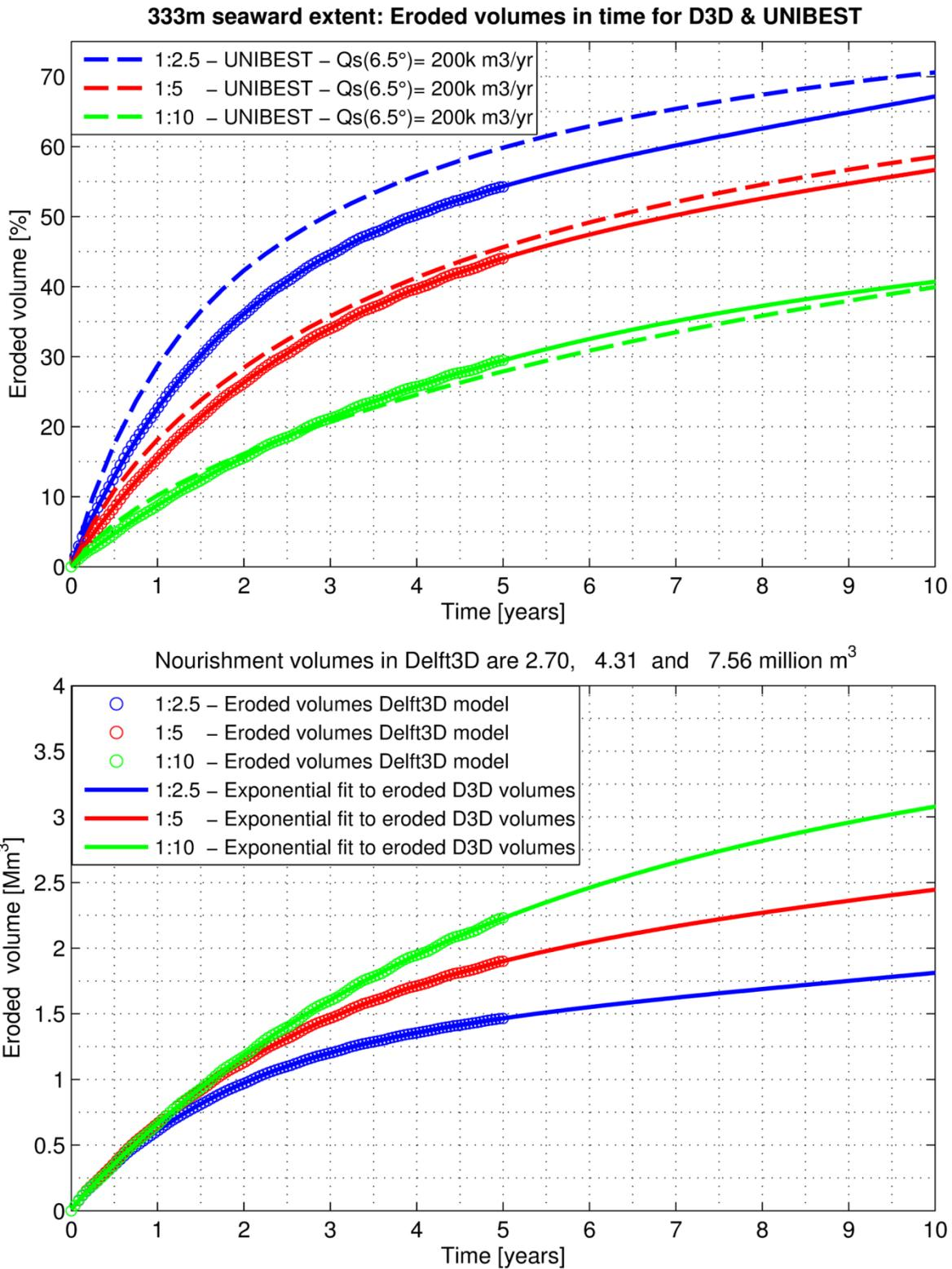
Figure G.2 – Eroded volumes in time for 333m seaward extent – D3D & UNIBEST
