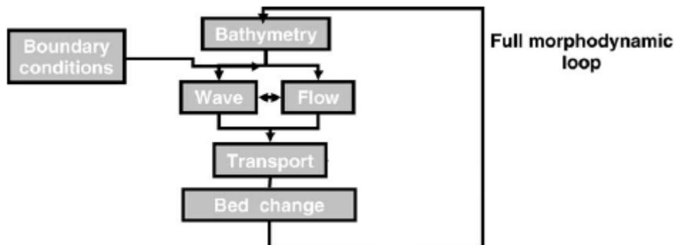
Figure B.1 – Flow diagram of Delft3D (Roelvink, 2006)
