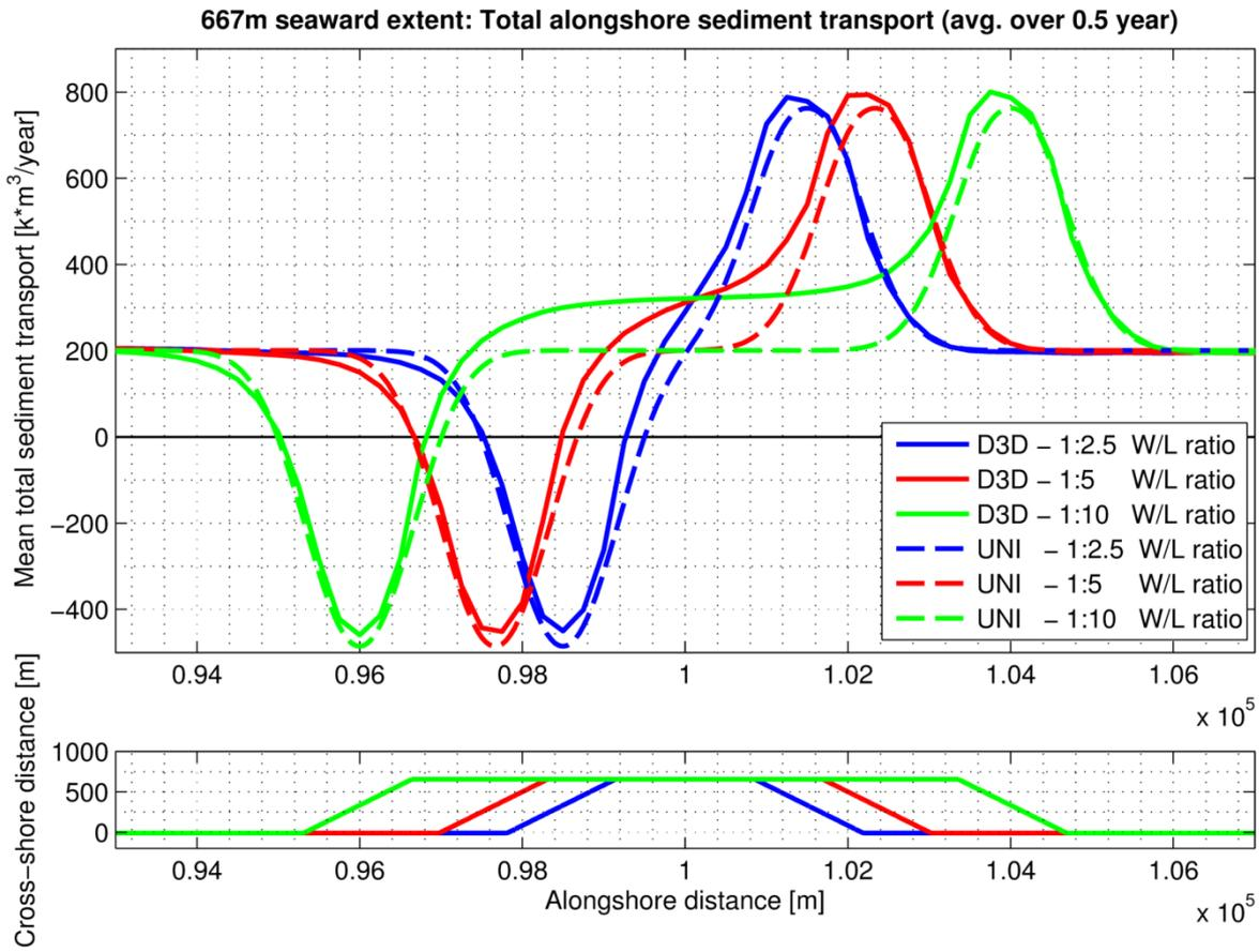
Figure G.6 – Net alongshore sediment transport plotted against the alongshore distance for the 667m seaward extent nourishments
