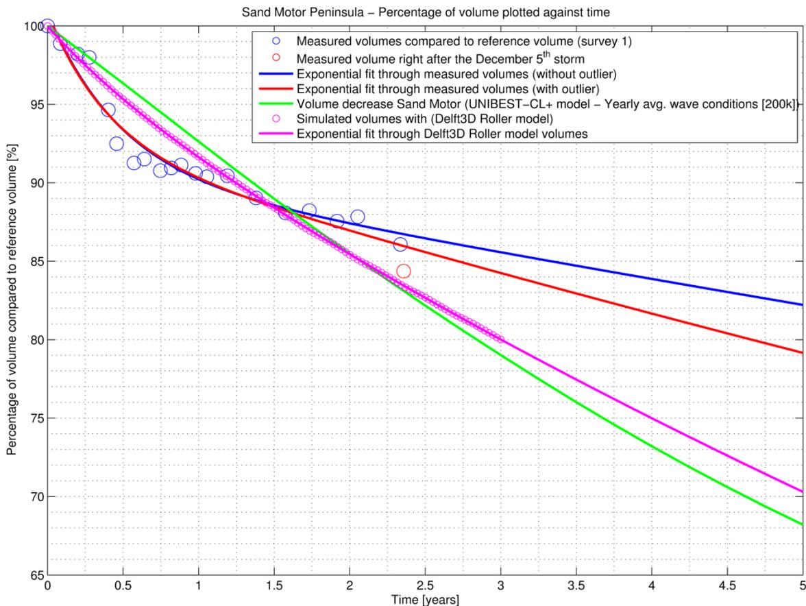
Figure 3.20 – Volume decay of Sand Motor (magenta coloured dots and line represent the Delft3D results)
