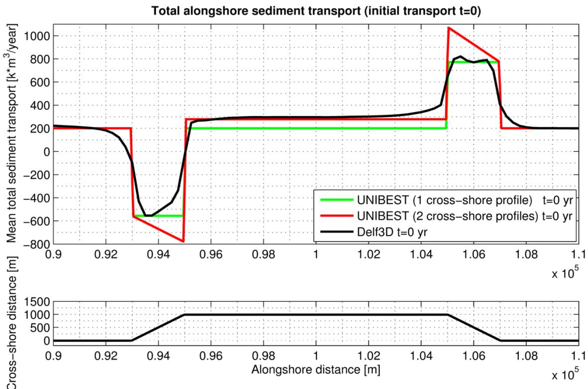
Figure 5.7 – Comparison of alongshore sediment transport for UNIBEST with 1 & 2 cross-shore profiles
