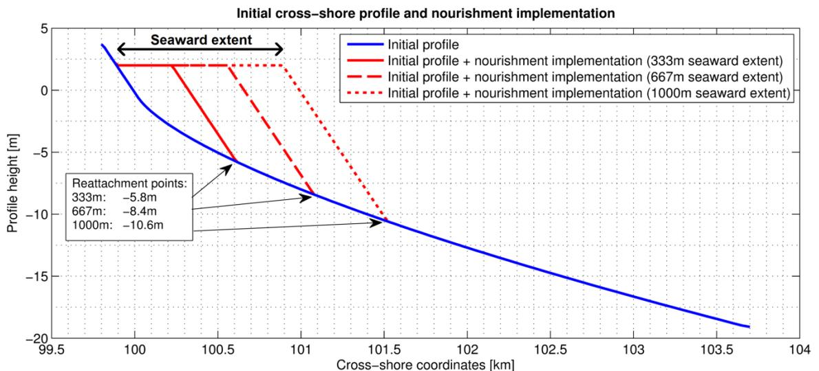
Figure 3.11 – Initial cross-shore profile and cross-shore profiles for the 333m, 667 and 1000m nourishments
