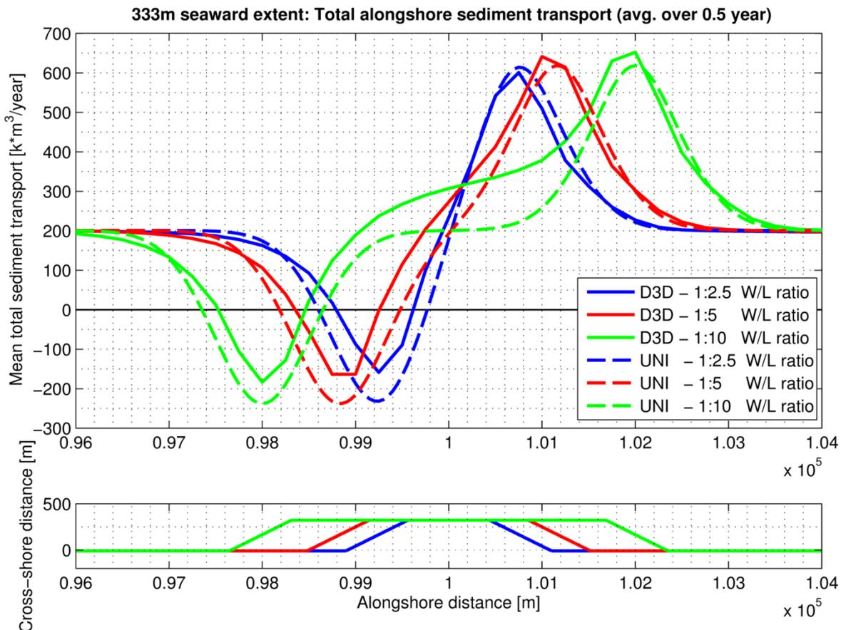
Figure 5.4 – Net alongshore sediment transport vs. alongshore distance for the 333m seaward extent nourishments
