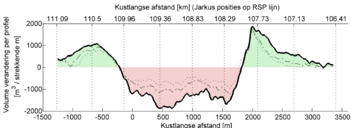
Figure 2.5 – Changes in volume plotted against the alongshore stretch of coastline: the dotted line represent the situation after 6 months, the dash-dot line the situation after 1 year and the solid line after 2 years. Red = erosion; green = accretion. (Shore Monitoring & Research, 2013)
