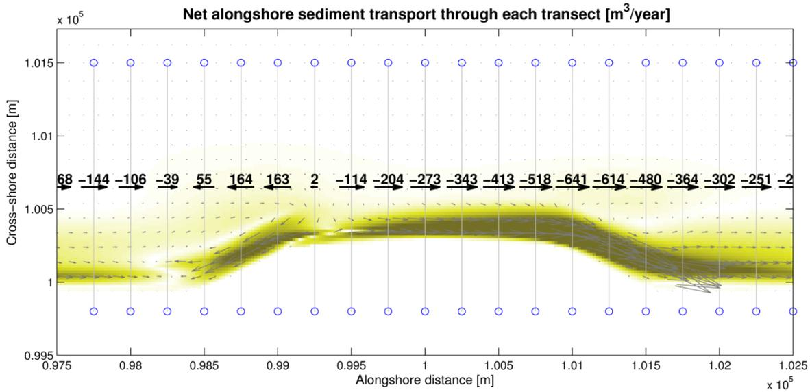
Figure 5.3 – Top view of 333m x 1665m nourishment with alongshore sediment transports through each transect
