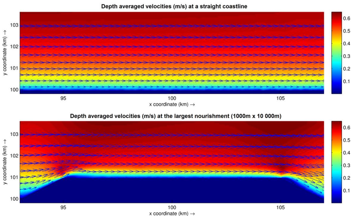
Figure 5.8 – Maximum depth averaged velocities (m/s) at a straight coastline and at the largest nourishment
