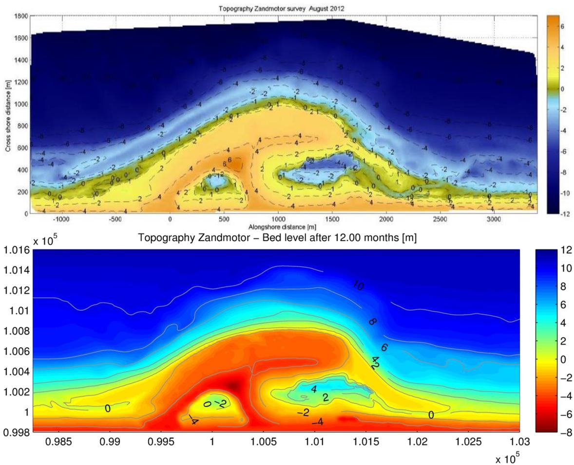
Figure 3.17 – Measured topography Sand Motor August 2012 (upper) and simulated topography Delft3D (lower).
