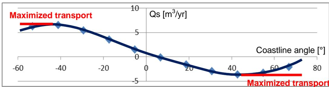
Figure 3.1 –  $S-\phi$  curve with forced maximum transports for relative wave angles larger than about 45 degrees
