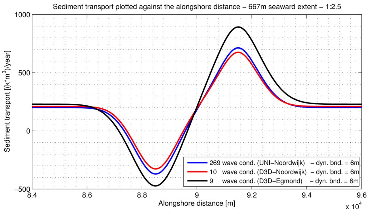
Figure 4.11 – Alongshore sediment transport at t=1 year for three different wave climates within UNIBEST
