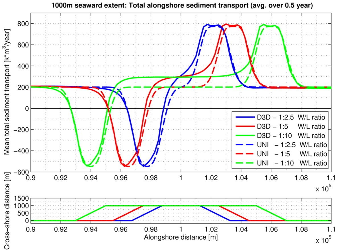
Figure G.9 – Net alongshore sediment transport plotted against the alongshore distance for the 1000m seaward extent nourishments
