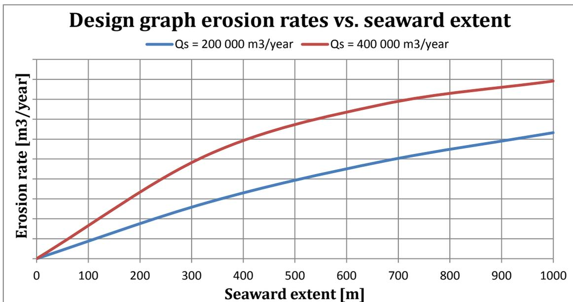
Figure 1.5 – Conceptual figure of erosion rates plotted against the seaward extent
