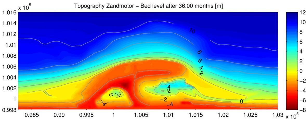
Figure C.3 – Van der Westhuysen expression –  $D_h = 1.00 \text{ m}^2/\text{s}$ : Topography Sand Motor after 36 months
