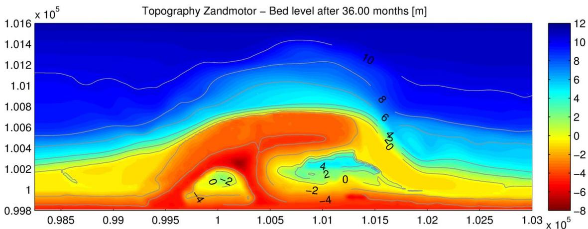
Figure C.2 – Van der Westhuysen expression –  $D_h = 0.25 \text{ m}^2/\text{s}$ : Topography Sand Motor after 36 months
