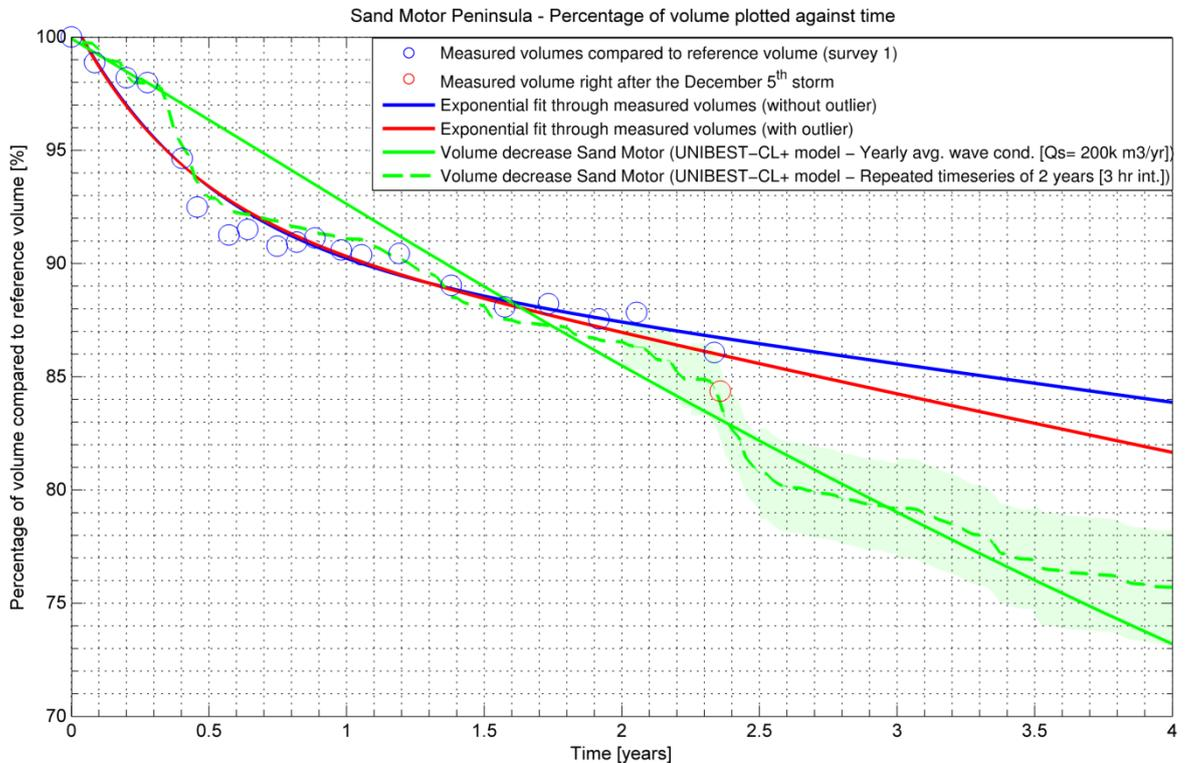
Figure 3.8 – Close-up of volume decay of Sand Motor (green lines are according to UNIBEST-CL+ model)
