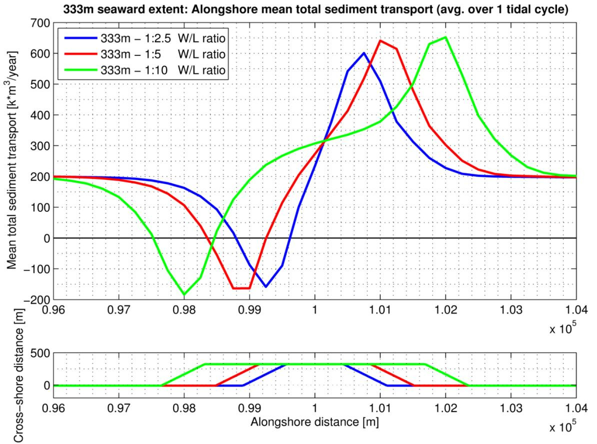
Figure G.3 – Net alongshore sediment transport plotted against the alongshore distance for the 333m seaward extent nourishments
