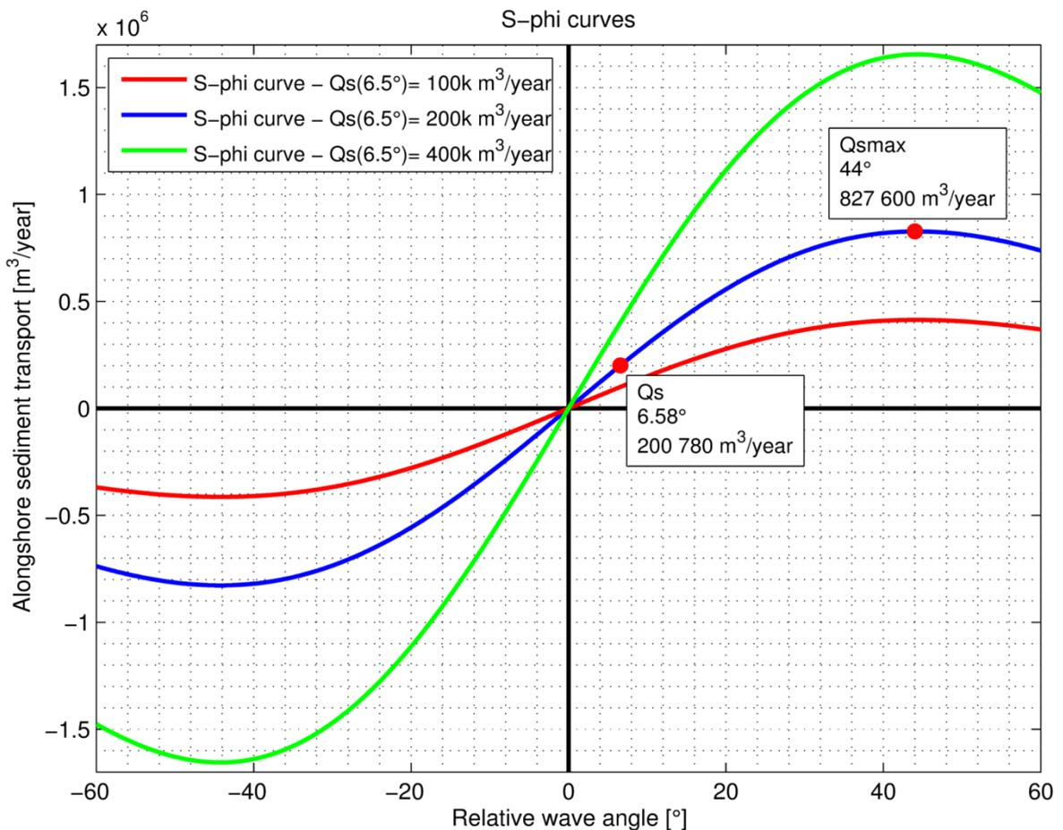
Figure 3.6 – Three different  $S-\phi$  curves used in the UNIBEST-CL+ calculations
