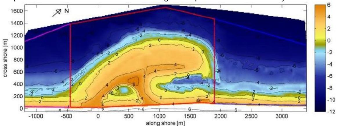
Figure 2.3 – Areas for which the volume calculations are carried out (red, blue and magenta polygons). (Shore Monitoring & Research, 2013)
