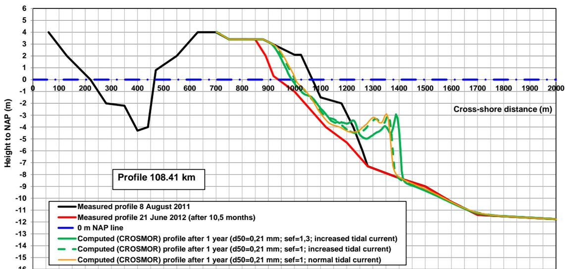
Figure D.3 – Measured and computed cross-shore profiles for ‘Jarkusraai 108.41’ (van Rijn, 2014a)
