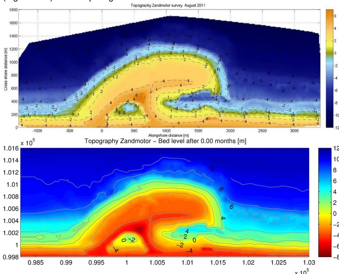
Figure 3.16 – Measured topography Sand Motor August 2011 (upper) and initial bathymetry Delft3D (lower). Upper figure from Shore Monitoring & Research (2013)
