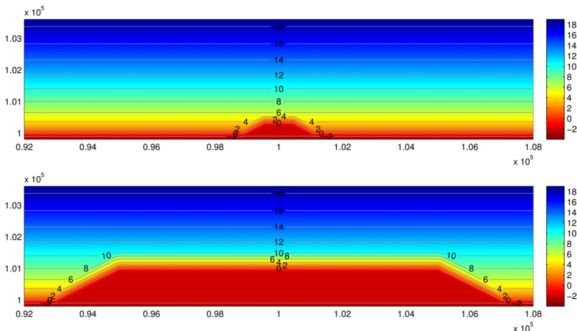
Figure 3.12 – Top view of bathymetry for smallest (333m x 833m) and largest (1 000m x 10 000m) nourishment
