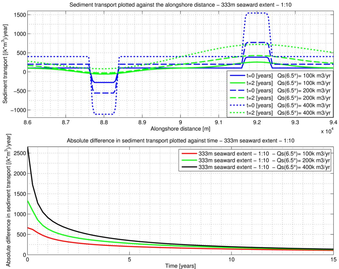
Figure 4.5 – Sediment transport in alongshore direction (upper) and in time (lower) for the 333m 1:10 nourishment
