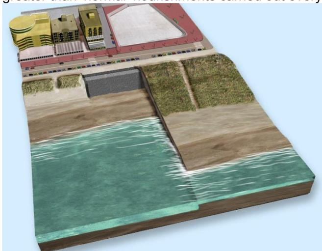
Figure E.5 – Impression of old situation (left) and new situation (right) (©Provincie Zuid-Holland)
