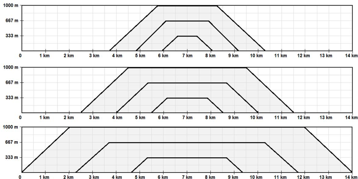
Figure 1.1 – Top view of nourishment dimensions. Upper plot: 1:2.5; Middle plot: 1:5; Lower plot: 1:10 (note that the x- and y-axis do not have the same scale!)
