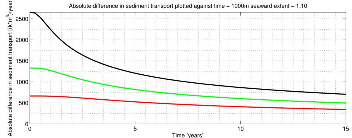
Figure F.12 – Sediment transport in alongshore direction (upper) and in time (lower) for the 1000m 1:10 nourishment
