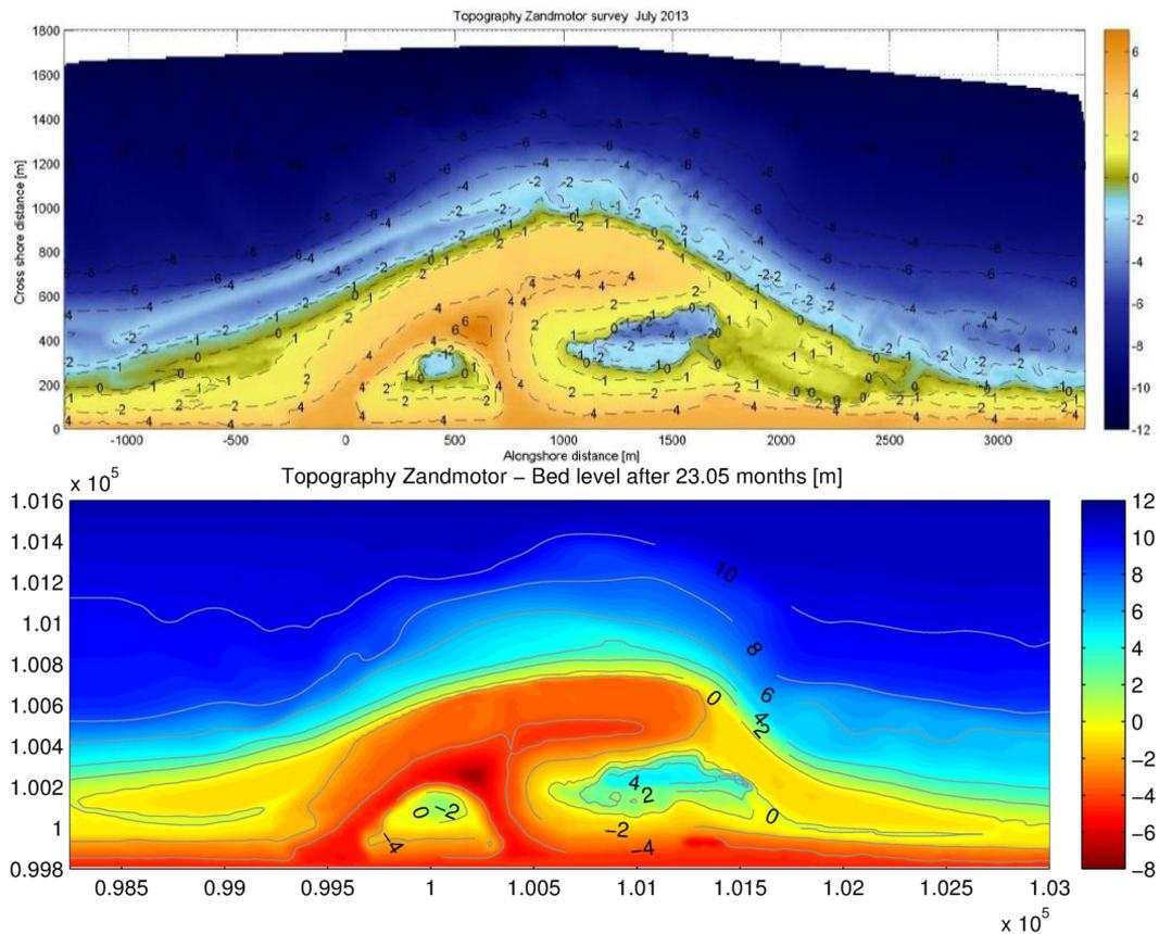
Figure 3.18 – Measured topography Sand Motor July 2013 (upper) and simulated topography Delft3D (lower). Upper figure from Shore Monitoring & Research (2013)
