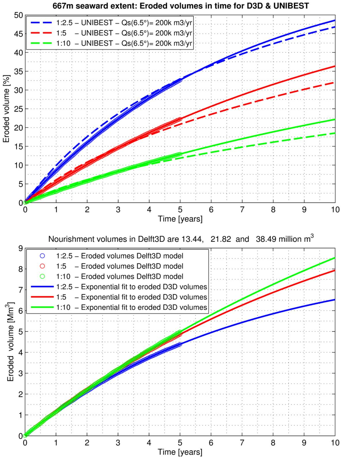
Figure G.5 – Eroded volumes in time for 667m seaward extent – D3D & UNIBEST
