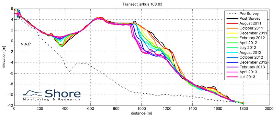
Figure D.1 – Cross-shore profiles for 'Jarkusraai' 108.83 located at the centre of the Sand Motor (Shore Monitoring & Research)
