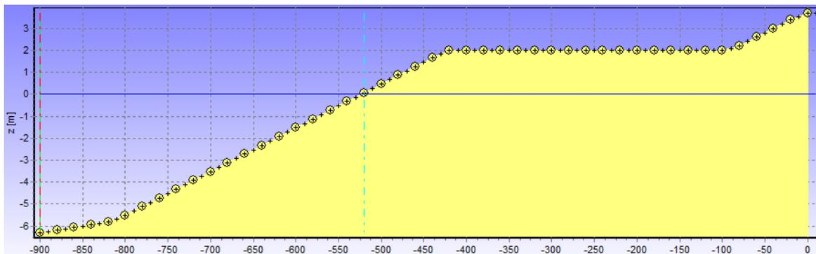
Figure 5.6 – Cross-shore profile for the nourishment section within UNIBEST
