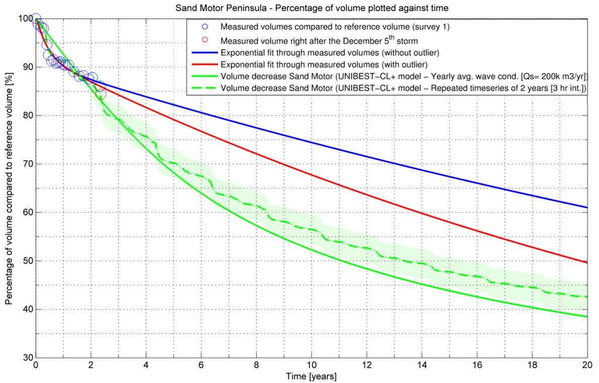
Figure 3.7 – Volume decay of Sand Motor (green lines are according to UNIBEST-CL+ model)
