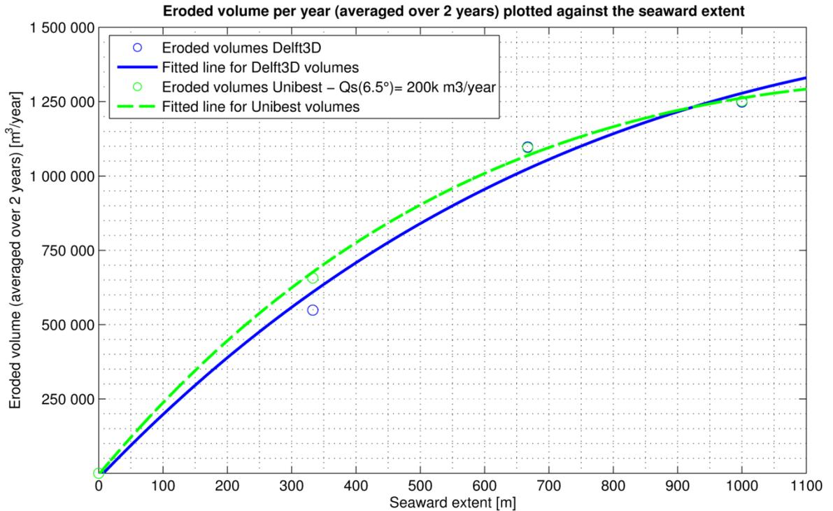
Figure 5.9 – Eroded volume per year (averaged over 2 years) plotted against the seaward extent – D3D & Unibest
