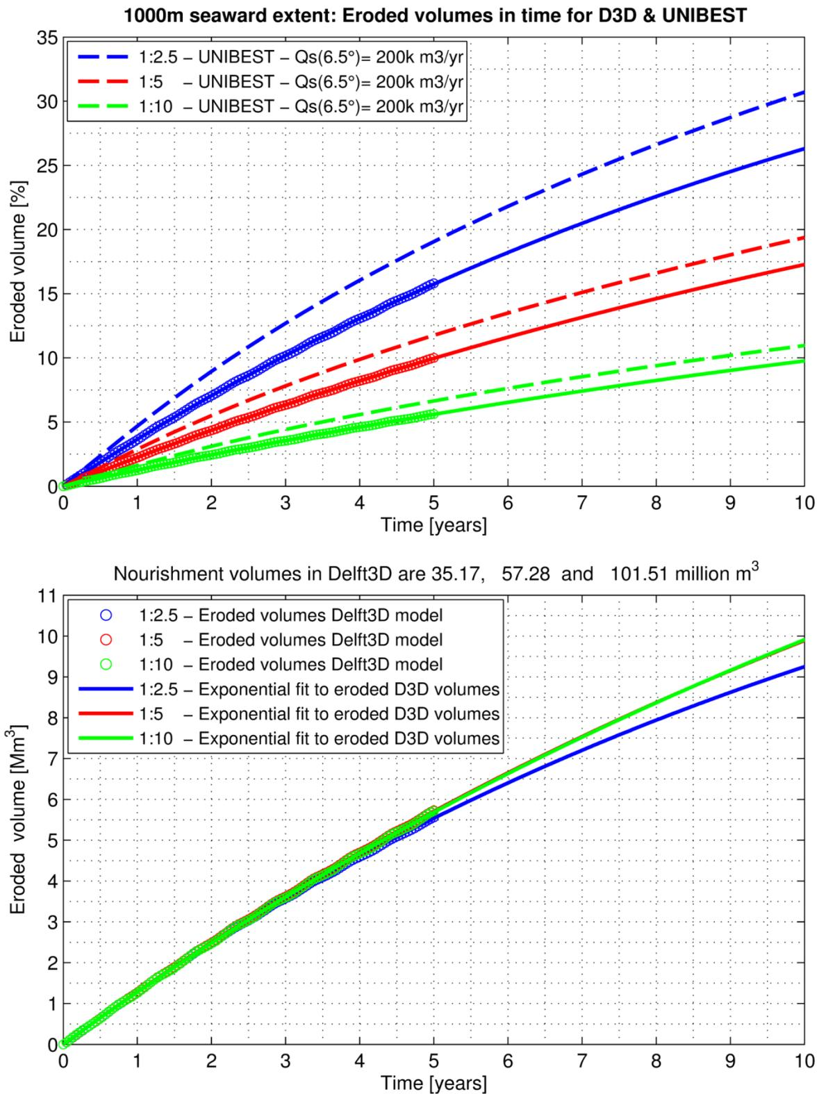
Figure G.8 – Eroded volumes in time for 1000m seaward extent – D3D & UNIBEST
