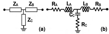
Fig. 4. Pad model using (a) T-shaped impedance equivalent and (b) lumped elements
