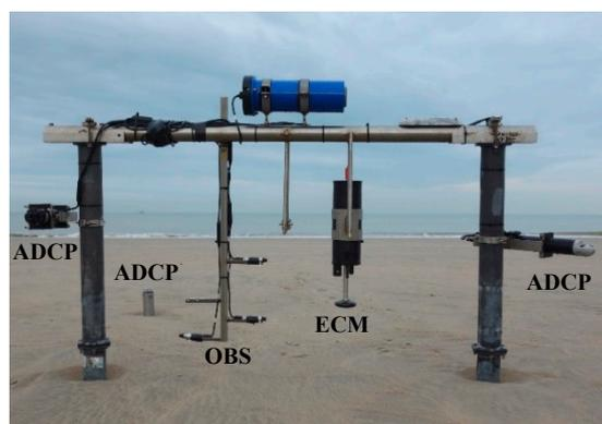
**Figure 2.** The intertidal measuring frame (1 m high, 2.2 m wide) with the down-looking Acoustic Doppler Current Profiler (ADCP), up-looking ADCP (not on the frame), three Optical Backscatter Sensors (OBS), Electromagnetic Current Meter (ECM), and up-looking ADCP.
